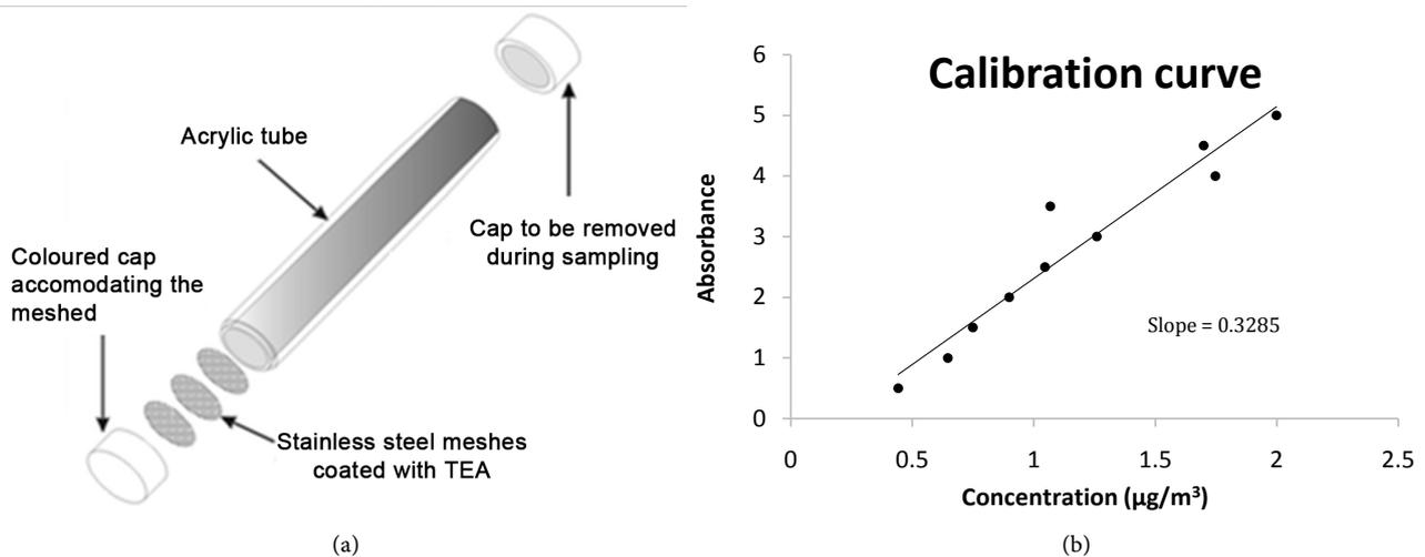
**Figure 1.** (a) Schematic of NO<sub>x</sub> diffusion tubes; (b) Calibration curve.
