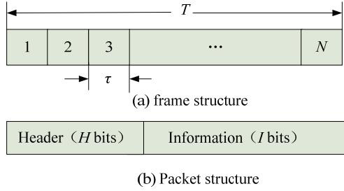
**Figure 2. Structure of frame and packet.**
