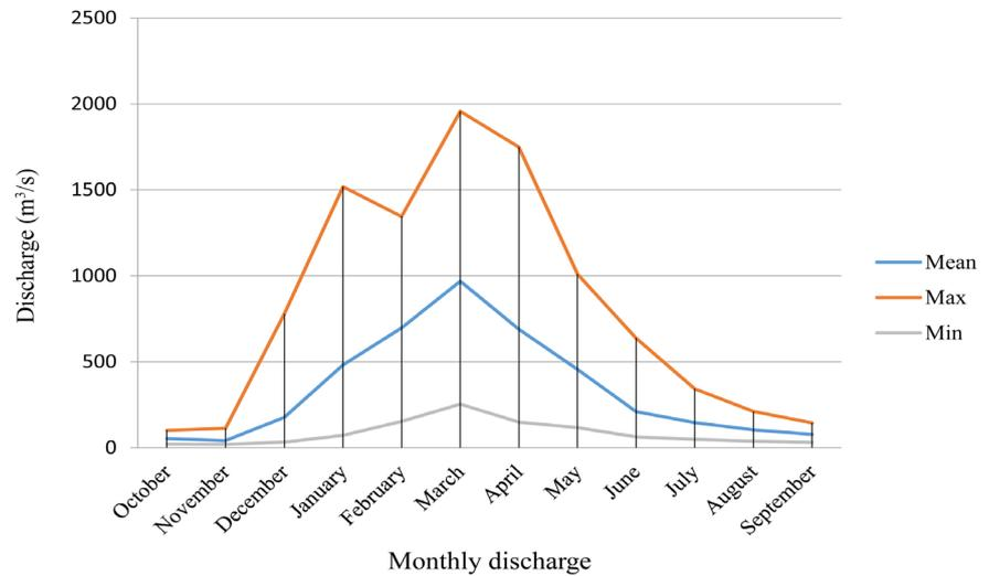
**Figure 1.** Kafue River hydrograph of unregulated water flows in cubic metres per second at Itetzitetzzi before the construction of the dam based on JICA (1992) and ZACPLAN (1994).
