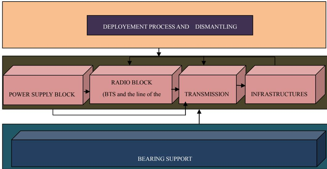
Figure 3. Synoptic presentation of a movable radio site.
