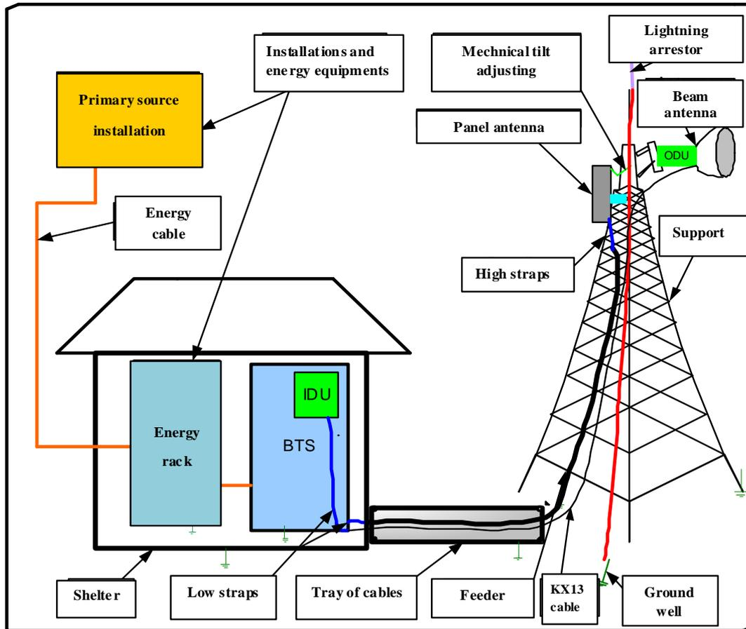
Figure 2. Architecture of an immobile radio site.
