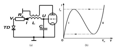
**Figure 1.** Scheme and volt-ampere characteristic of an electronic generator with a nonlinear tunnel diode.
