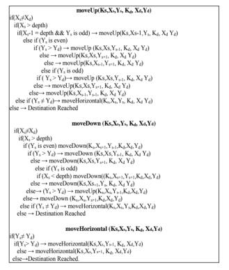
Figure 6. Routing algorithm for MLH(k,d).
