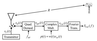
Figure 1. Block diagram of monostatic radar using complex stretch processing.
