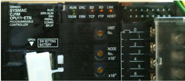
Figure 11. PLC ethernet module light indicator status.
