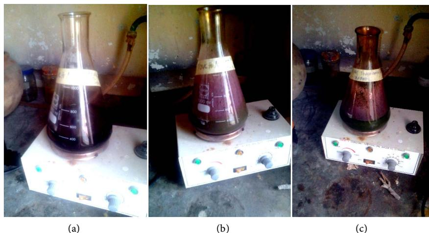
**Figure 1.** (a) Mixture of graphite flakes,  $\text{H}_2\text{SO}_4$  and  $\text{KMnO}_4$  at the onset of stirring; (b) Resulting mixture after three days of stirring; (c) Resulting mixture after six days of stirring.
