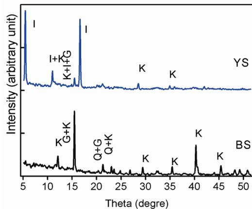
**Figure 2.** The DRX pattern of the crude soils used showing the Bragg peaks of the major mineral elements. K = Kaolinite; I = Illite; G = Goethite ( $\alpha$ -FeOOH); Q = Quartz; BS = Brazzaville soil; YS = Yengola soil.
