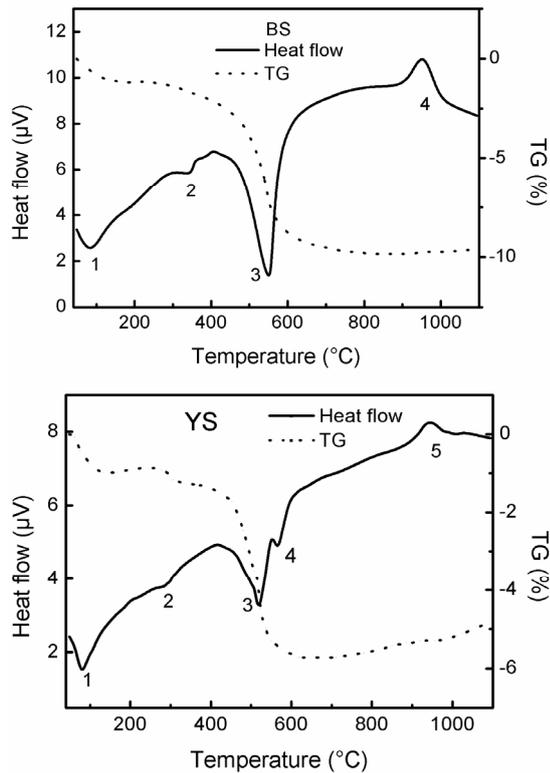
**Figure 3.** Thermal analysis of the crude soils exhibiting characteristic endothermic and exothermic peaks of clays: 1) Dehydration; 2) decomposition of goethite and organic matter; 3) Kaolinite dehydroxlation; 3) Illite dehydroxylation; 4) restructuration of metakaolinite.
