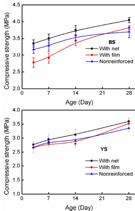
**Figure 4.** Variation of the compressive strength with the time and the reinforcement of the CEBs made with the press of 6 MPa.
