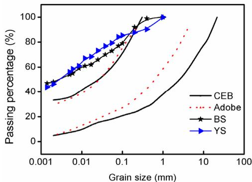
**Figure 1.** Grading grain size curves of the two soils compared to the standards grading curves for CEB and adobe.
