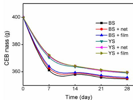
**Figure 6.** Effect of the reinforcement on the drying kinetics of CEBs.
