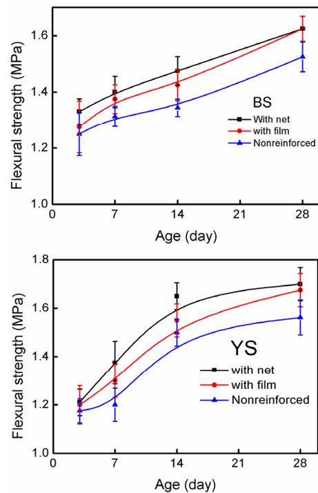
**Figure 5.** Variation of the flexural strength with the time and the reinforcement of the CEBs made with the press of 6 MPa.
