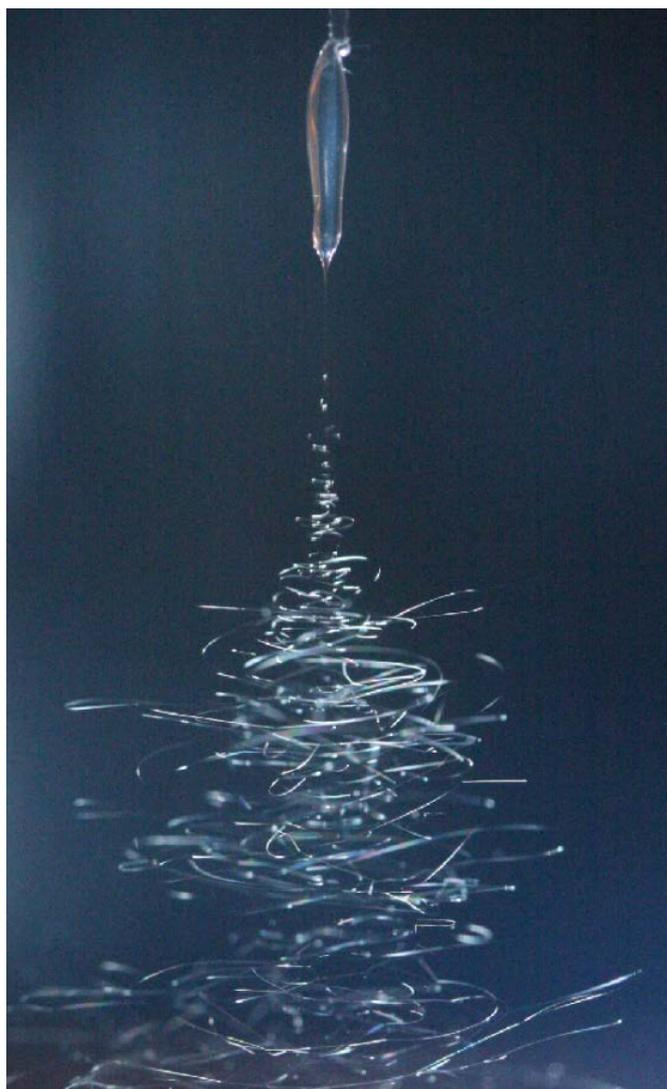
**Figure 1.** Ideal electrospinning process.
