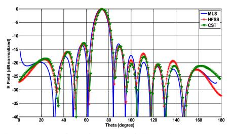
Figure 3. Comparison of patterns by MLS, HFSS and CST at 5.35 GHz.
