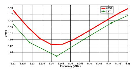
Figure 4. Diagram of VSWR Simulated by HFSS and CST softwares.
