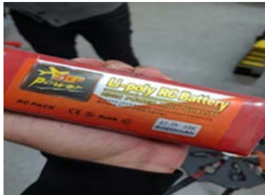
Figure 2. Selected batteries: Selecting a battery that can supply the appropriate voltage for the EDF output ( 400\text{ g} \times 2 = 800\text{ g} ).
