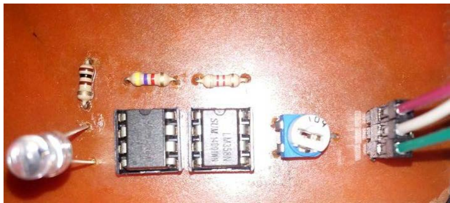
Figure 10. Components soldered on receiver PCB.
