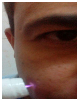
Figure 4. Human face contacting with the nitrogen-plasma jet without any electrical shock.
