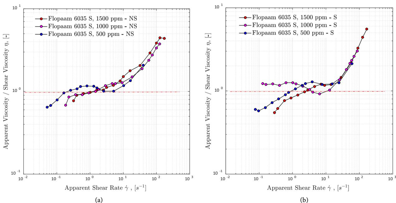
**Figure 10.** Ratio between apparent viscosities measured in Bentheimer core plugs and Bulk viscosity by fitting the Carreau-Yasuda model plotted against the apparent shear rate corrected by rheometer data. The data plotted is for the HPAM Flopaam 6035 S, non-sheared (a) and pre-sheared (b) in a 4 g/l TDS brine solvent.
