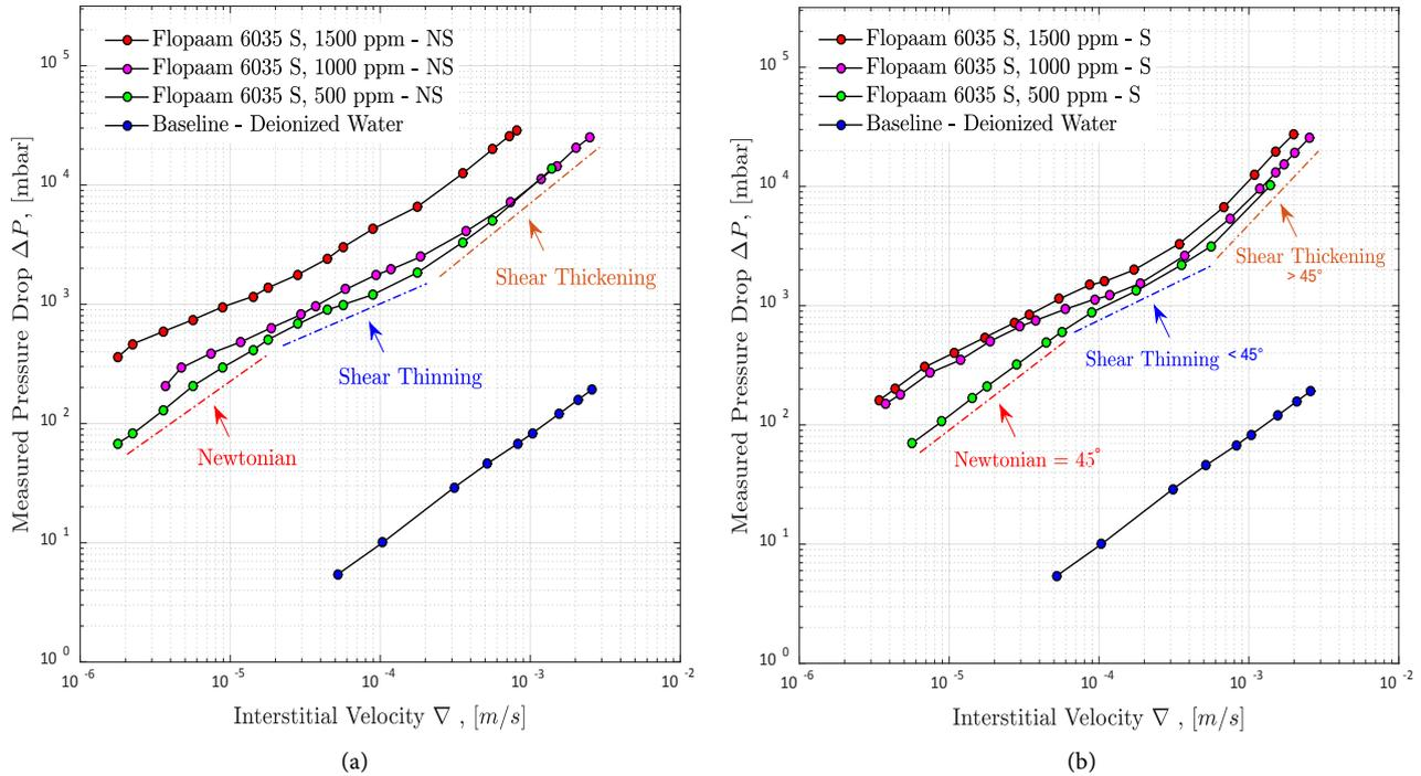
**Figure 5.** Measured pressure drop as a function of interstitial velocity for an HPAM solution through a Bentheimer core plug. The data plotted is for the HPAM Flopaam 6035 S, non-sheared (a) and pre-sheared (b) at different concentrations in a 4 g/l TDS brine solvent. Pressure data plotted is the one recorded during the experiment by flooding polymer solutions for different injection rates.
