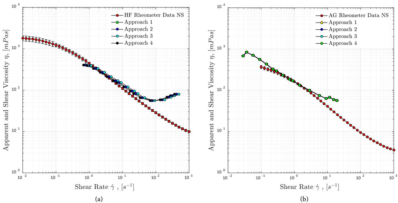
**Figure 7.** Apparent flow curves obtained by relating the bulk viscosity to core flooding. The data shown belong to a Hengfloc 63026 1500 ppm non-sheared in a 4 g/l TDS brine solvent (a) and a biopolymer Actigum CS6 1500 ppm non-sheared in a 4 g/l TDS brine solvent (b).
