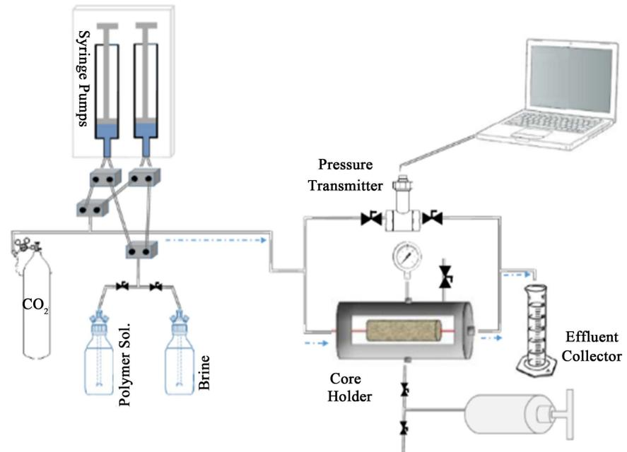
**Figure 3.** Sketch of core flood experimental setup. It is connected via PTFE Teflon tubing and stainless steel pipes to the syringe pump and a differential pressure gauge.
