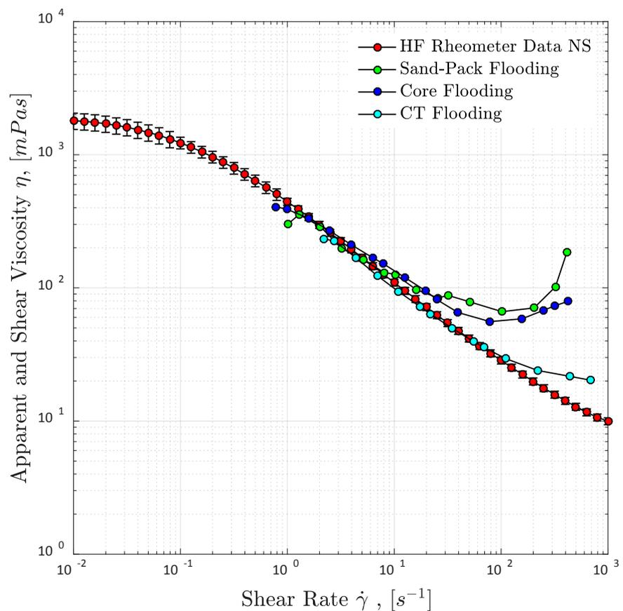
**Figure 8.** Apparent flow curves obtained by relating the bulk viscosity to core flooding, sand-pack and capillary tube injection. The data shown belongs to a Hengfloc 63026 1500 ppm non-sheared in a 4 g/l TDS brine solvent. Approach 1 is used for apparent shear rate calculation.
