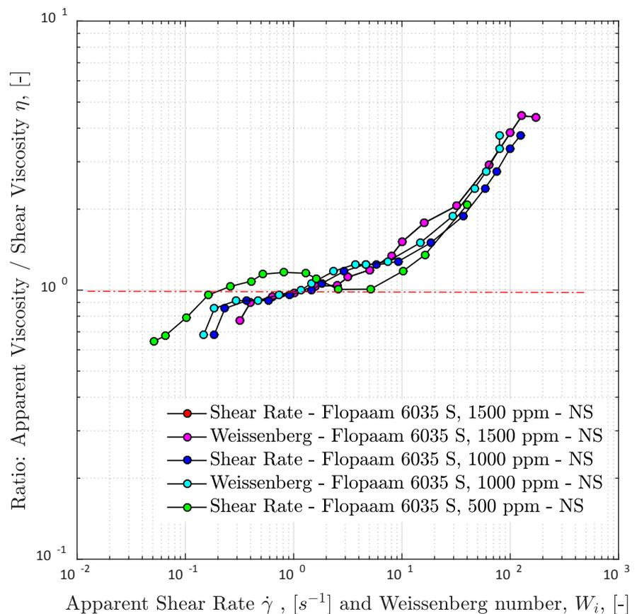
**Figure 11.** Ratio between apparent viscosity measured in Bentheimer core plugs and bulk viscosity by fitting the Carreau-Yasuda model plotted against the apparent viscosity corrected by rheometer data as well as Weissenberg number. The data plotted is for the HPAM Flopaam 6035 S, non-sheared at different concentrations in a 4 g/l TDS brine solvent.
