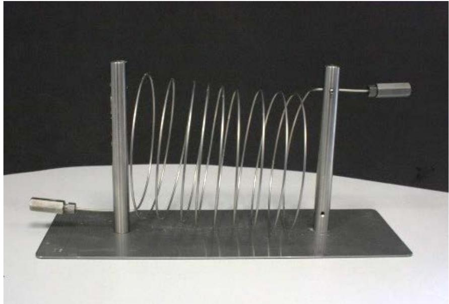
**Figure 4.** Stainless steel capillary tube (CT) setup. Designed to compare apparent viscosity in core flood and sand-pack flood (impact of converging-diverging geometry).
