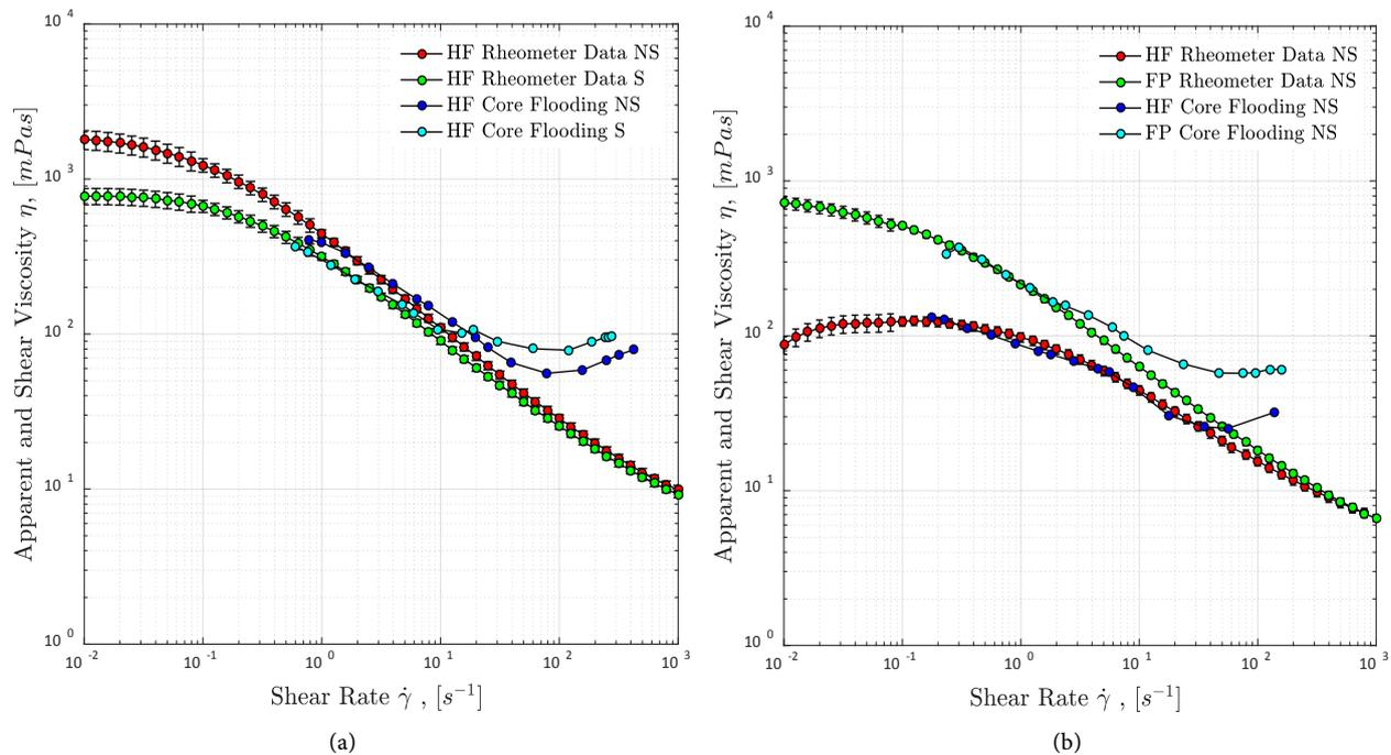
**Figure 9.** Apparent flow curves obtained by relating the bulk viscosity to core flooding. The data shown on (a) belong to a Hengfloc 63026 1500 ppm non-sheared/sheared in a 4 g/l TDS brine solvent. The data shown on (b) belong to a Hengfloc 63026 1000 ppm non-sheared and Flopaam 6035 S 1000 ppm non-sheared in a 4 g/l TDS brine solvent. Approach 1 is used for apparent shear rate calculation.
