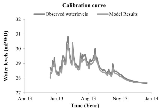
**Figure 2.** Calibration of Water level data at taluk-simulbari station for the year 2013.
