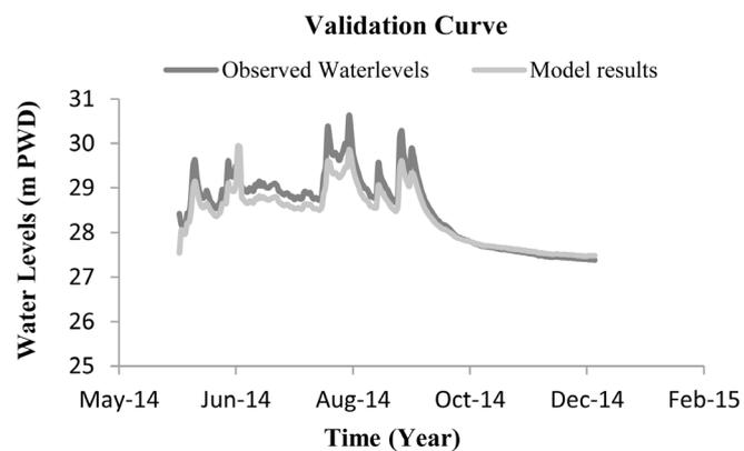
**Figure 3.** Validation of water level data at taluk-simulbari station for the year 2014.
