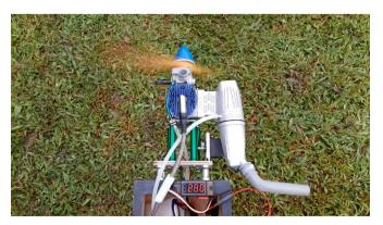
Figure 3. The test engine running on isopropanol.
