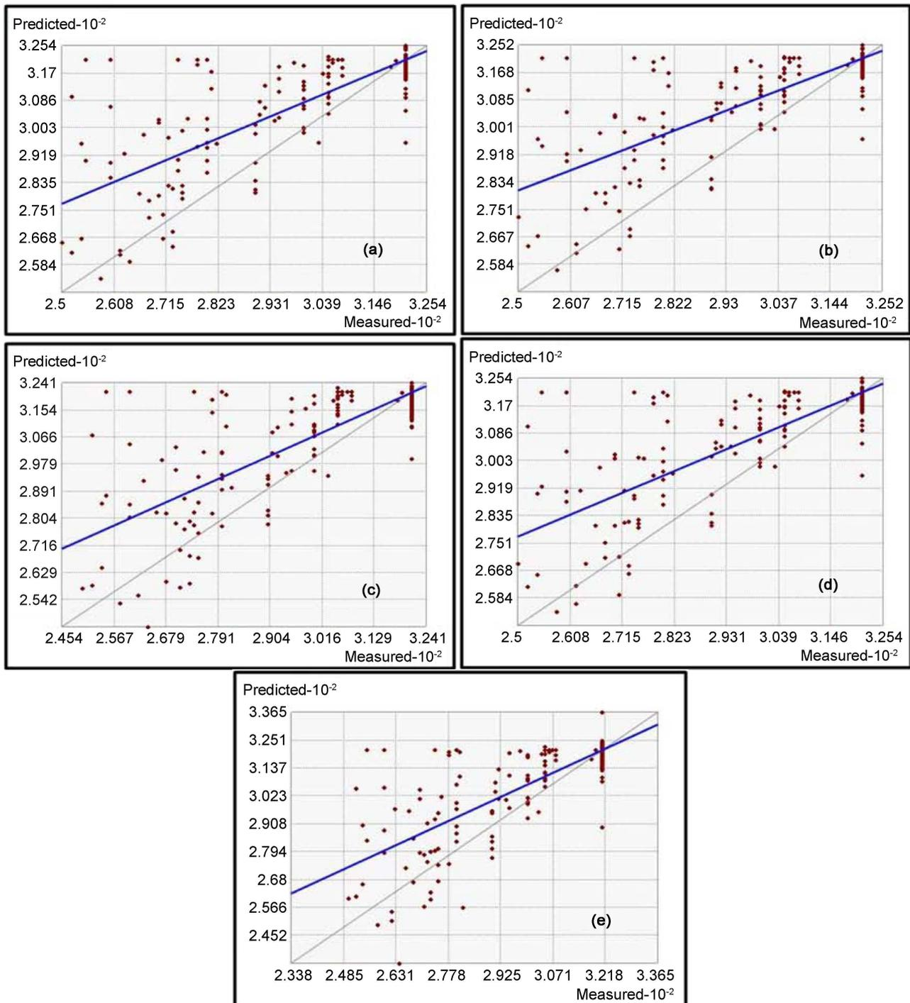
**Figure 5.** Comparison of the cross-validation (predicted vs. measured depth) of Mosul Lake by ordinary kriging models: (a) circular, (b) exponential, (c) Gaussian, (d) spherical and (e) stable (the blue line is the fitted line and black lines represent a perfect fit 1:1).
