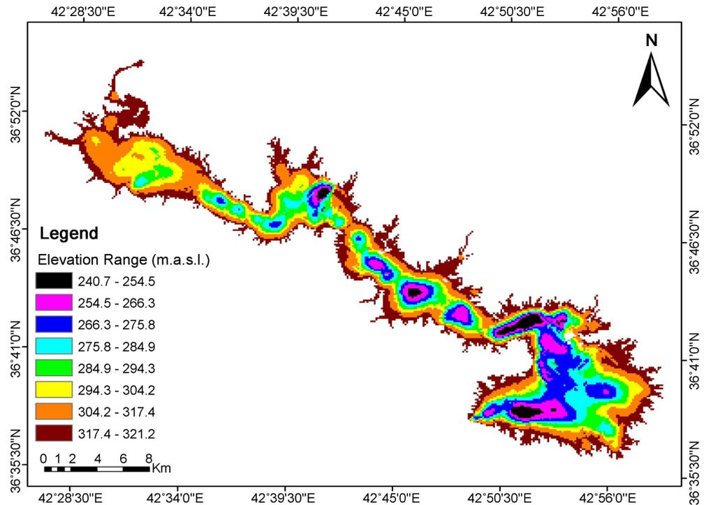
**Figure 4.** Bathymetric map of Mosul Dam Lake determined using the ordinary kriging interpolation method.
