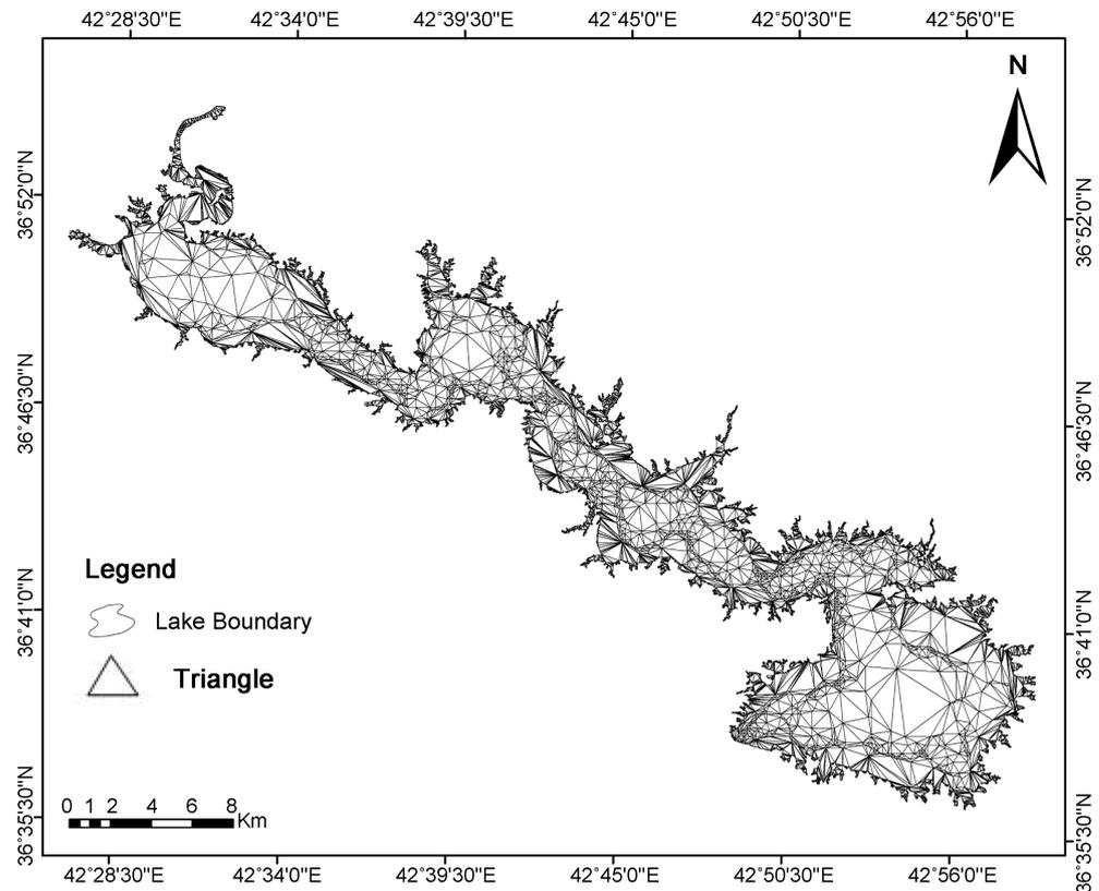
**Figure 3.** Subdivision of the lake into Delaunay triangles using the TIN approach for generating a digital bathymetric model of the study area.
