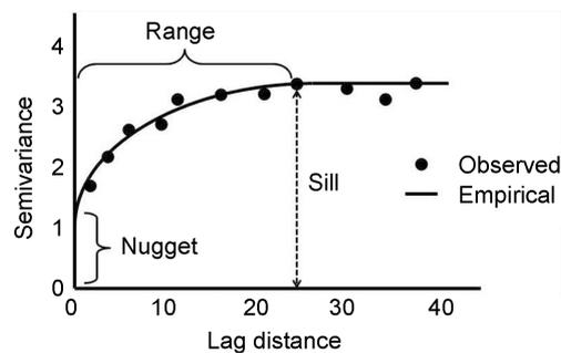
**Figure 6.** A theoretical example of semivariogram model showing different components [35].
