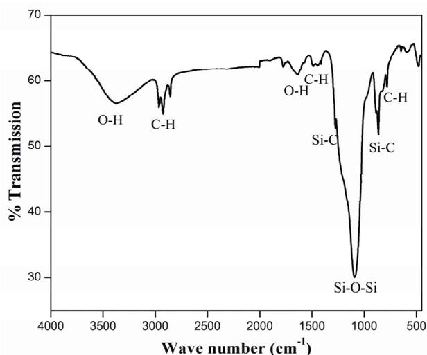
Figure 3. FTIR spectra of silica aerogel before absorption of solvents and oils.
