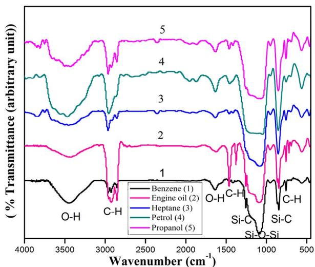
Figure 4. FTIR spectra of silica aerogel after desorption of solvents and oils.
