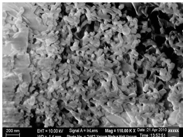
Figure 5. FESEM image of the aerogel before absorption of oil or organic liquids.
