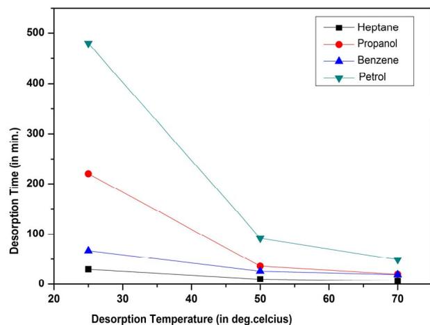
**Figure 2.** Desorption rate of TEOS based silica aerogels at different temperatures.
