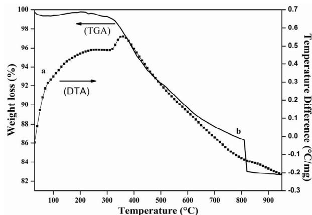
Figure 6. Thermo gravimetric and differential thermal analysis (TG-DTA) of aerogels.
