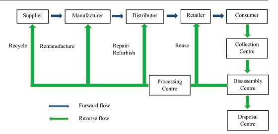
Figure 3. Closed-loop flow [11].
