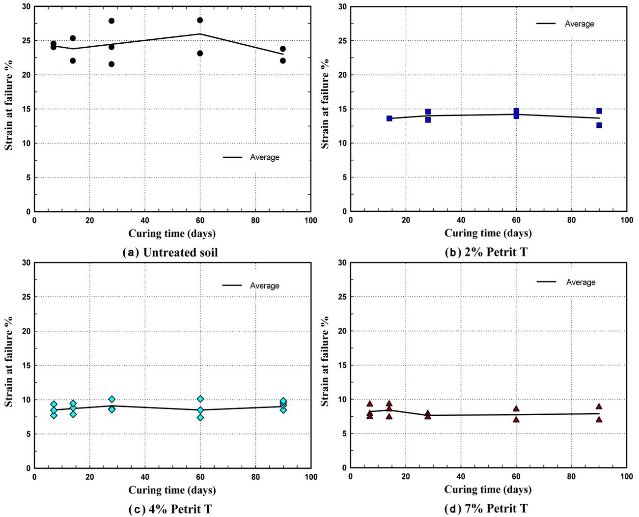
Figure 16. Strain at failure versus curing time and Petrit T content for all tests.
