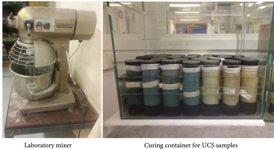
**Figure 2.** Laboratory mixer and curing specimens prepared for UCS and consistency limits tests.
