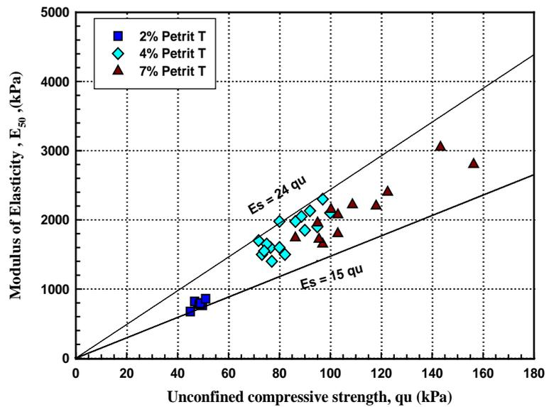
Figure 19. Modulus of elasticity versus UCS strength for different binder contents and length of curing periods.
