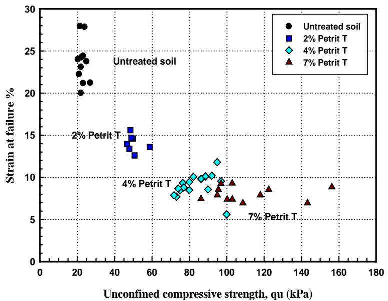
Figure 17. Strain at failure versus UCS strength.
