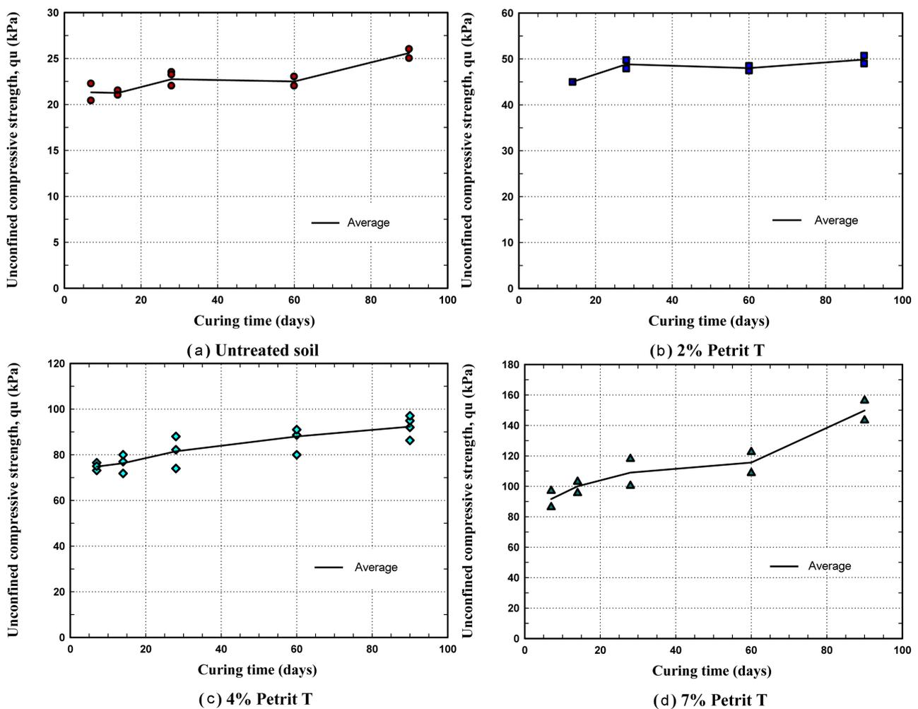
**Figure 13.** Unconfined compression strength versus curing time for different Petrit T content for all tests.
