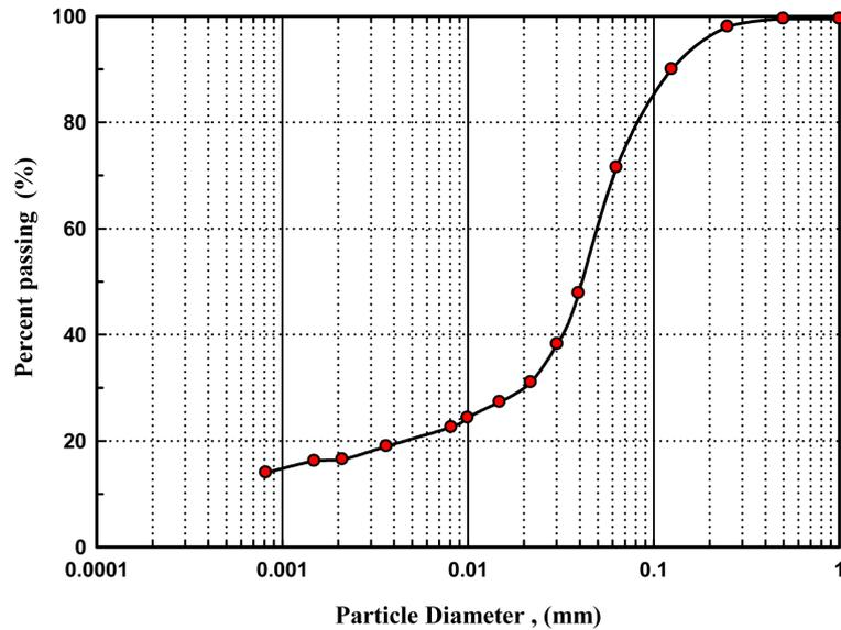
**Figure 1.** Particle size distribution of the untreated soil.
