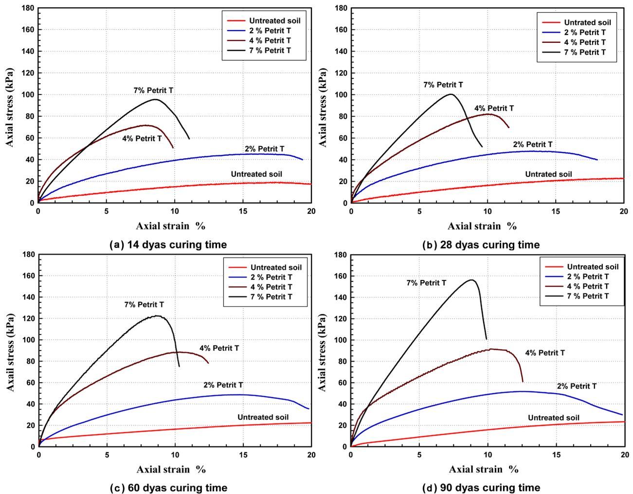
Figure 15. Stress-strain curves for untreated and treated soil with different Petrit T contents and curing time.
