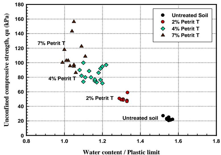
**Figure 14.** UCS versus water/plastic limit ratio for all tests.
