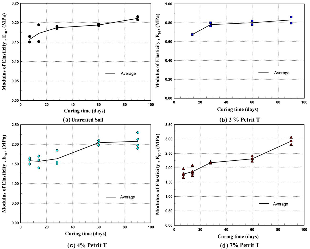
Figure 18. Modulus of elasticity versus curing time and binder content for all tests.
