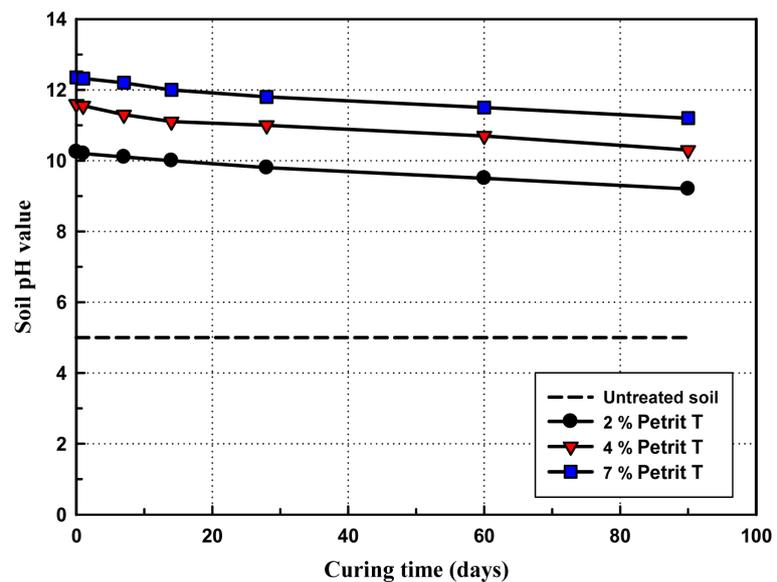
**Figure 12.** Effect of curing time and Petrit T content on the pH value of treated soil.
