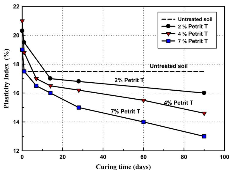
**Figure 4.** Effect of curing time and Petrit T content on plasticity index.
