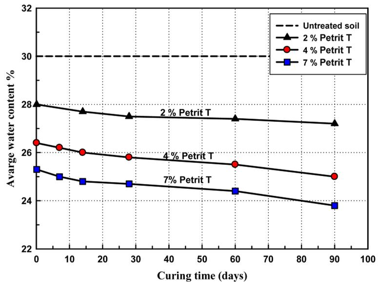
Figure 6. Effect of curing time and Petrit T content on water content.
