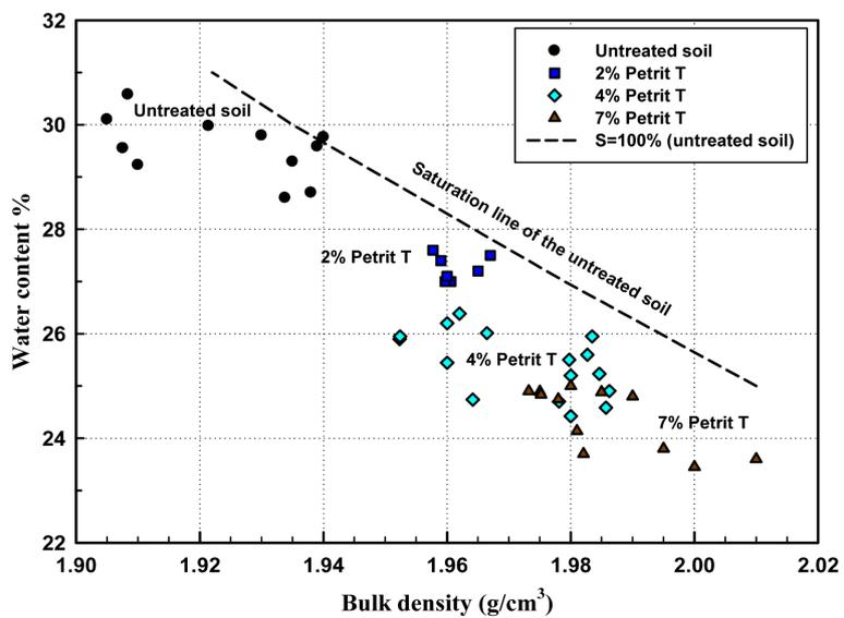
**Figure 10.** Specimen water content versus bulk density and Petrit T content for all curing time.
