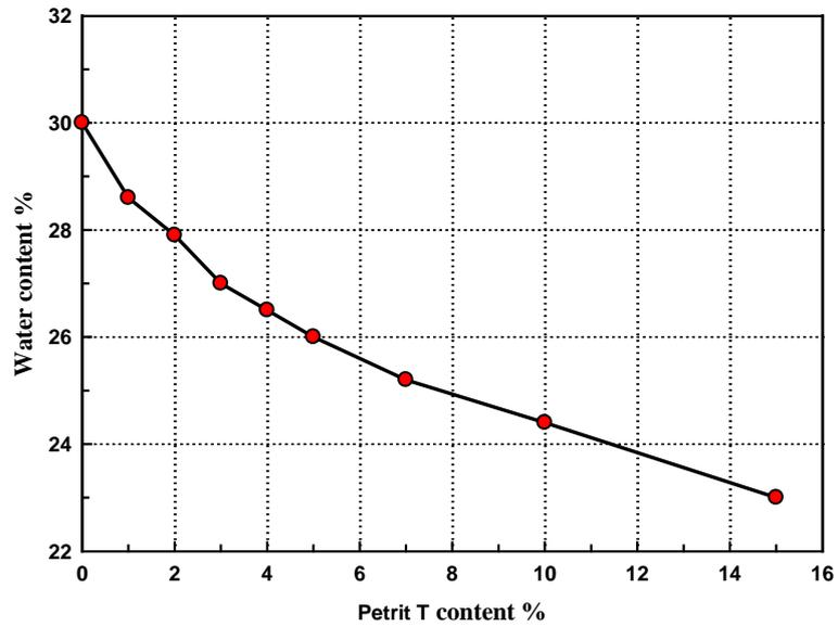
Figure 5. Immediate reduction in water content versus Petrit T content.
