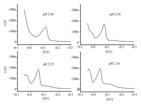
Figure 4. Potentiometric curves showing the effect of acidity on CAA +  $UO_2$  electrolyte.
