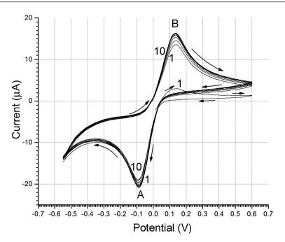
**Figure 3.** Cyclic voltammetry curves of chloranilic acid in presence of uranium drop (around 50  $\mu$ g/L), pH~3, acidified with H<sub>2</sub>SO<sub>4</sub>, over a SPE electrode (Metrohm E110), using carbon as working electrode and counter-electrode and silver as reference electrode. The numbers at the curves indicate the cycle repetition, where 1 is the first and 10 the last.
