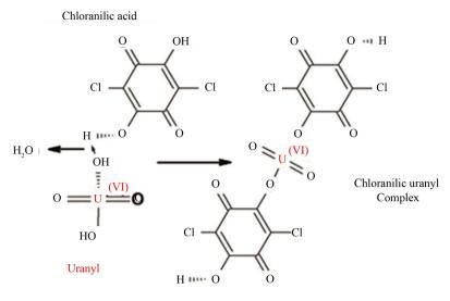
Figure 5. Schematic indication of the reaction of CAA and uranyl Complex.
