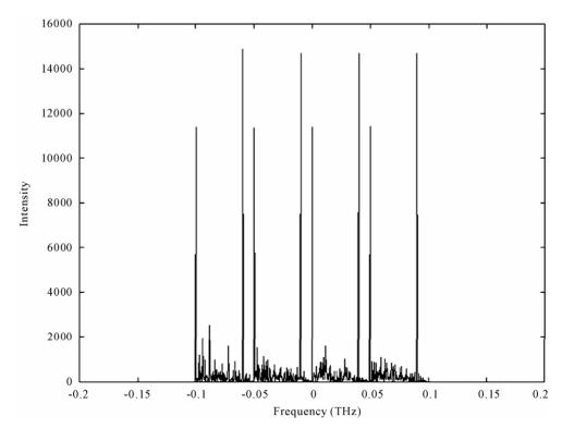
Figure 3. Signals' spectra using Gaussian filter with 48 GHz bandwidth.
