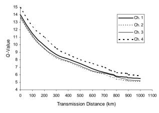
Figure 4. *Q*-value versus propagation distance for all channels using peak power = 3 mW and FWHM = 6 ps. (Channels' definitions: Ch. 1 = 1554.4 nm; Ch. 2 = 1554.8 nm; Ch. 3 = 1555.2 nm; Ch. 4 = 1555.6 nm).
