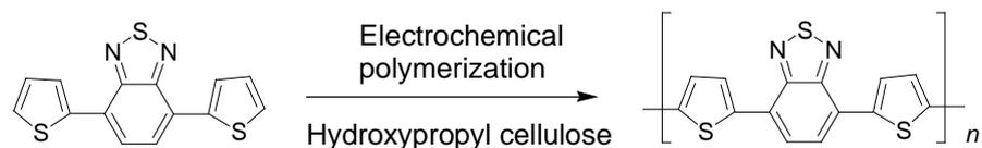
**Figure 1.** Scheme of electrochemical polymerization of [thiophene]-[benzo[1,2,3]thiadiazole]-[thiophene] monomer in hydroxypropyl cellulose.
