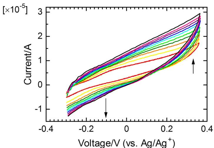
**Figure 9.** Cyclic voltammograms of P(T-Btdaz-T)/HPC composite at various scan rates of 10, 20, 30, 40, 50, 60, 70, 80, 90, and 100 mV/s vs. Ag/Ag<sup>+</sup>.
