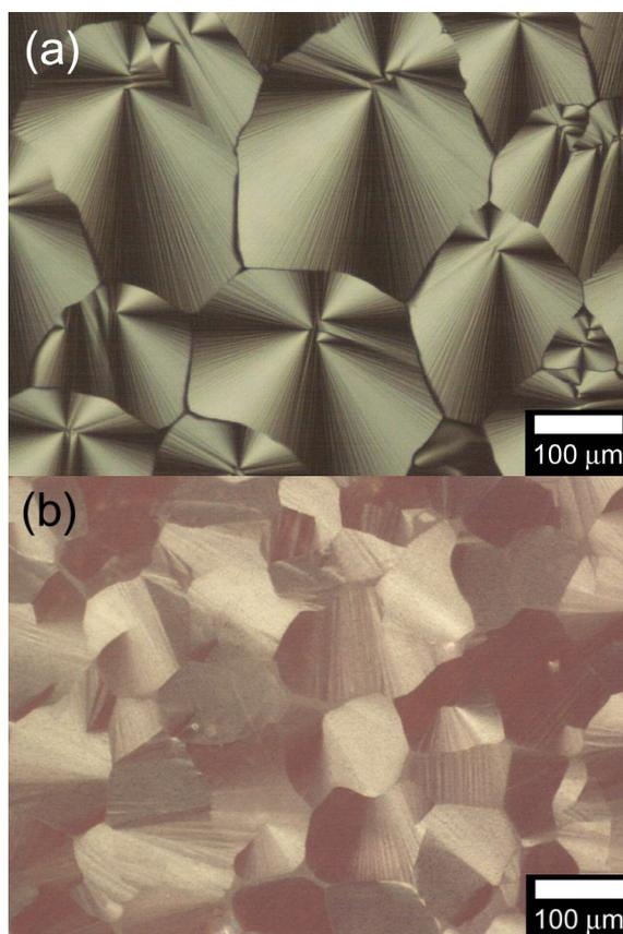
**Figure 4.** Polarizing optical microscopy image of columnar liquid crystal electrolyte solution (a) and polymer film (b) prepared by columnar phase.
