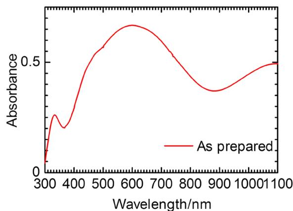
**Figure 8.** UV-vis absorption spectrum of PEDOT film prepared in columnar liquid crystal electrolyte solution.
