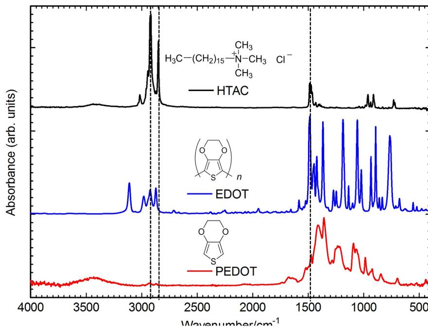
**Figure 6.** Fourier transform infrared spectra of hexadecyltrimethylammonium chloride (HTAC) (black line), EDOT (blue line) and PEDT (red line).
