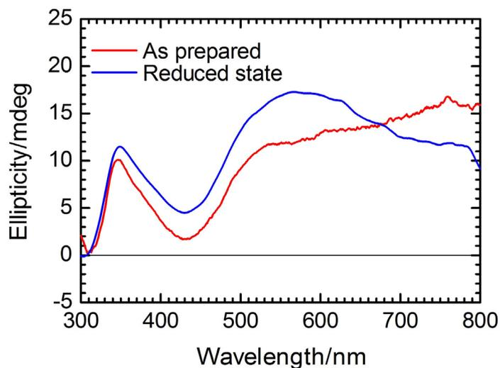
**Figure 11.** CD spectra of P(T-Btdaz-T)/HPC composite. (Red line): as prepared sample. (Blue line): reduced state.
