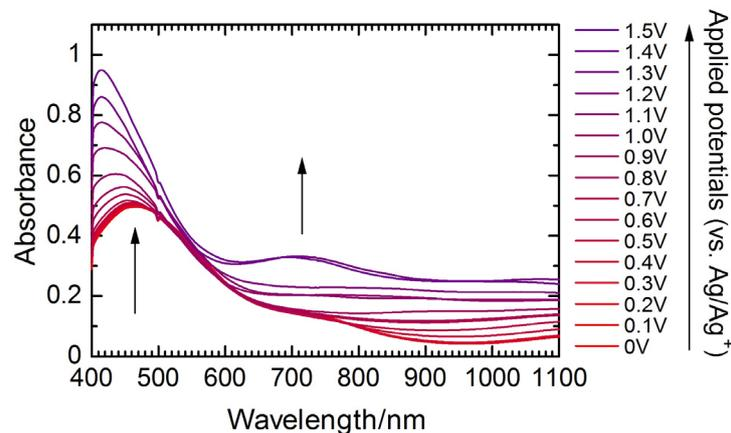
**Figure 7.** UV-vis absorption spectra of P(T-Btdaz-T)/HPC composite at various applied potentials (vs. Ag/Ag<sup>+</sup>).
