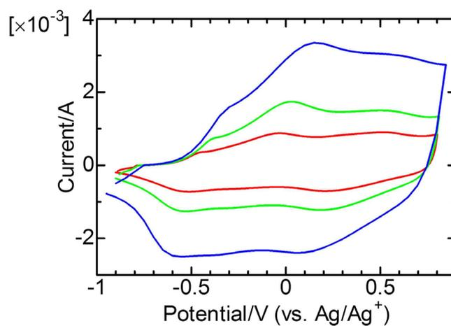
**Figure 10.** Cyclic voltammograms of PEDOT prepared in HPC polymer liquid crystal at various scan rates of 100, 200 and 500 mV/s vs. Ag/Ag<sup>+</sup>.
