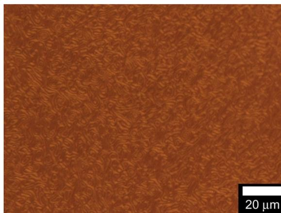
**Figure 3.** Polarizing optical microscopy image of obtained polymer film P(T-Btdaz-T) in hydroxypropyl cellulose (HPC).
