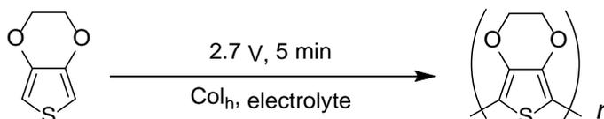
**Figure 2.** Electrochemical polymerization of 3,4-ethylenedioxythiophene in columnar liquid crystal.
