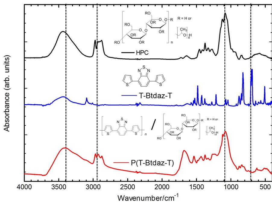
**Figure 5.** Fourier transform infrared (IR) spectra of hydroxypropyl cellulose (HPC) (black line), T-Btdaz-T (blue line), and resultant polymer (P(T-Btdaz-T)/HPC) composite, red line).
