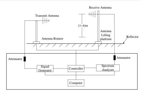
Figure 1. AF measurement system.
