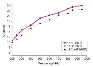
Figure 4. AF of log-periodic antennas calibrated.
