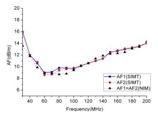
Figure 3. AF of biconical antennas calibrated.
