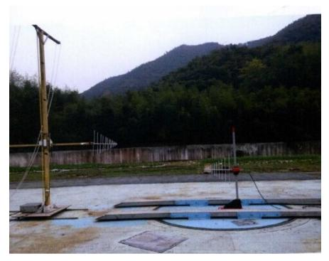
Figure 2. AF measurement system on OATS.
