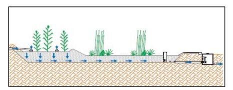
Figure 1. Cross-Section of the purification Bed of a Pure Reedbed STS [26].
