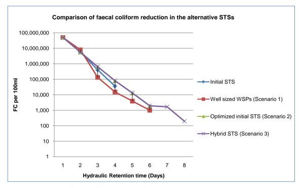
Figure 4. Comparison of faecal coliform reduction in the alternative STSs.
