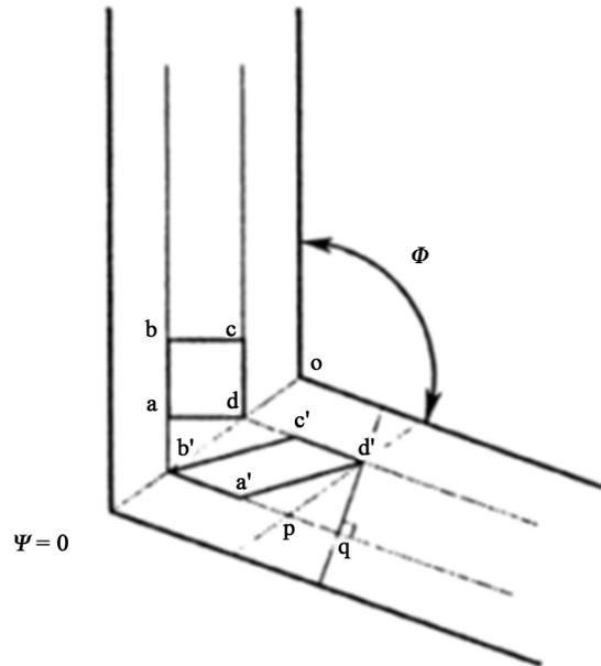
**Figure 1.** Schematic diagram showing the extrusion principle for SPD: two sequential channels, which intersect at an angle  $\Phi = 120^\circ$  and  $\psi = 0^\circ$ , which defines the arc of curvature of the junction (Valiev, 2000).
