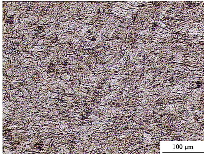
**Figure 7.** Optical micrograph of the nickel alloy 600 after heat treatment of 673 K during 1800s also after four ECAP passes, presence of elongated grains and precipitates identified by EDS microanalysis-SEM, electron and x-rays diffraction results.
