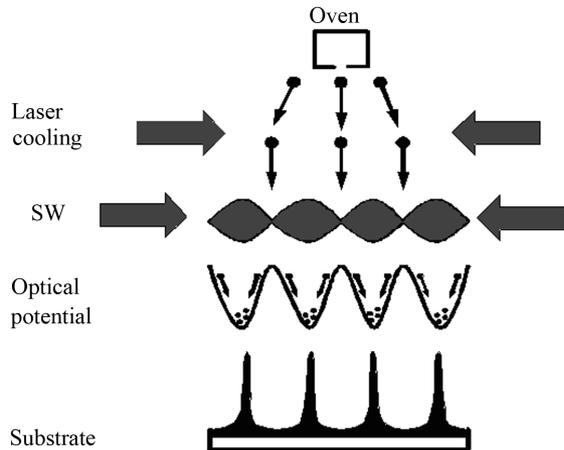
**Figure 1. Principle of laser focused Cr atomic deposition nano-grating structure.**
