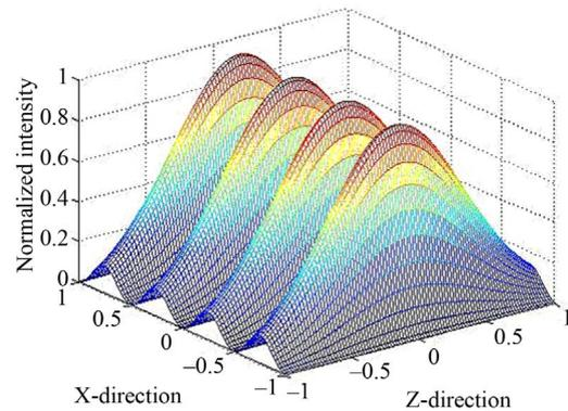
**Figure 2. Normalized intensity of Gaussian laser standing wave field.**
