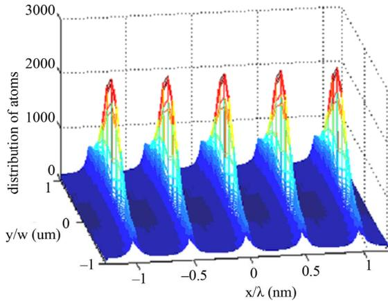
**Figure 5. Three dimensional stripes of Cr atom under ideal conditions.**
