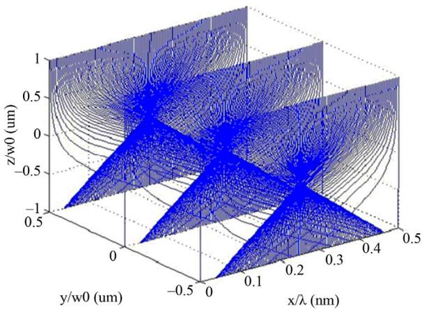
**Figure 8. Trajectories of chromium atoms under the influence of chromatic aberration.**
