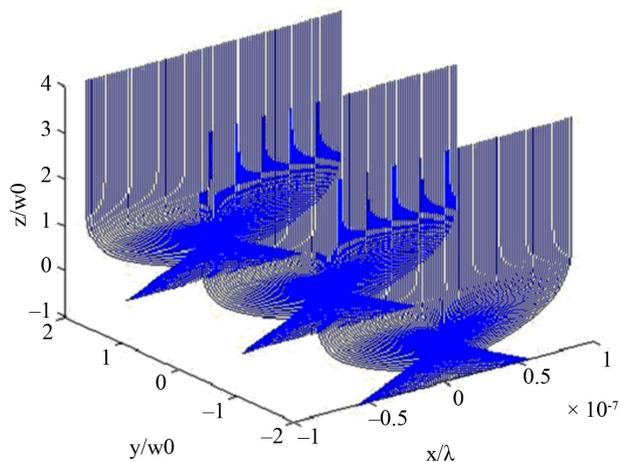
**Figure 10. Trajectories of chromium atoms under the influence of spherical aberration.**
