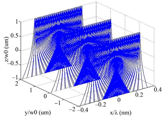
**Figure 6. Trajectories of chromium atoms under the influence of atomic beam divergence.**
