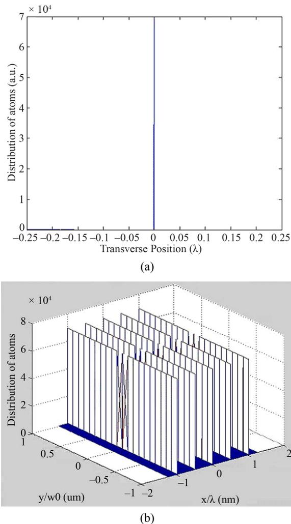
**Figure 11. (a) Deposition distribution of chromium atoms under the influence of spherical aberration; (b) Three dimensional stripes of chromium atoms under the influence of spherical aberration.**
