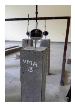
Figure 1. Shrinkage measurement.
