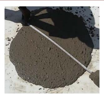
Figure 3. Flow of concrete for slump flow test.
