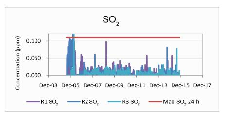
Figure 8. Monitoring data for sulphur dioxide from the three stations (R1, R2, R3).
