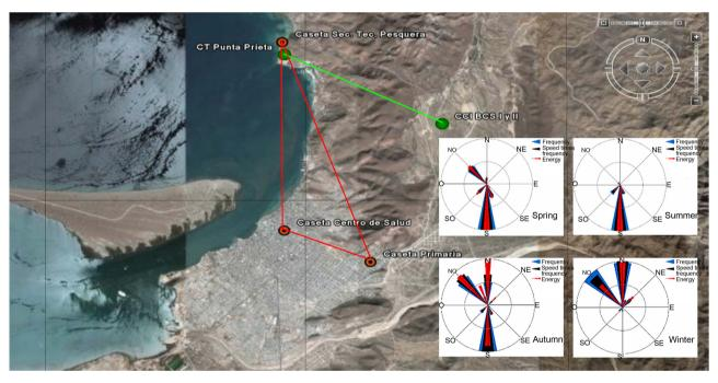
**Figure 7.** Location of air quality monitoring stations. Source: (CFE, 2008). Red dots correspond to monitoring stations (R1 at the top of the image, R2 directly South from R1 and R3 to the East of R2) and green dots correspond to power stations. The wind rose insets show prevailing wind directions in autumn (top left), winter (top right), spring (bottom left) and summer (bottom right).
