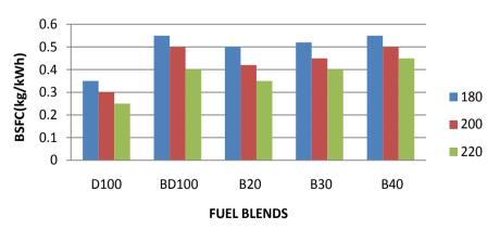
Figure 4. Brake specific fuel consumption at different IOP.
