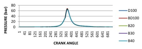
Figure 9. Cylinder pressure with CA at 200 bar IOP.
