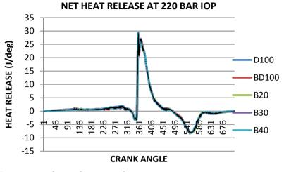
Figure 21. Net heat with CA at 220 bar IOP.
