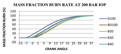
Figure 13. Variation of mass fraction burn with crank angle at 200 bar.
