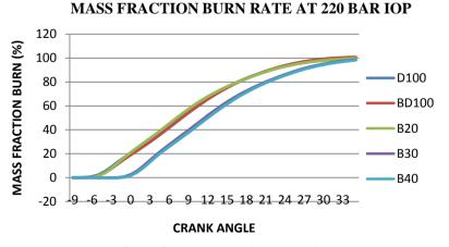
Figure 14. Variation of mass fraction burn with crank angle at 220 bar.
