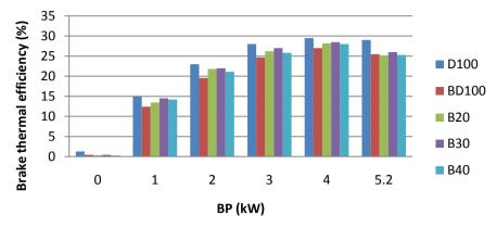
Figure 1. Brake thermal efficiency with BP.
