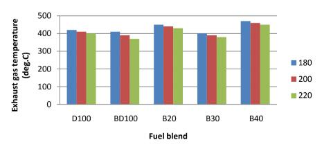
Figure 6. Exhaust gas temperature at different IOP.
