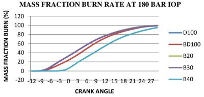
Figure 12. Variation of mass fraction burn with crank angle at 180 bar.
