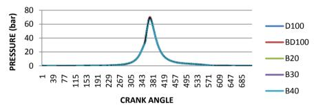
**Figure 7.** Cylinder pressure with crank angle.
