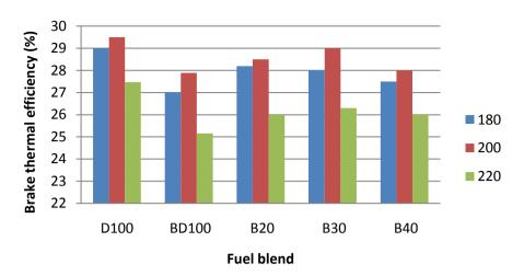
Figure 2. Brake thermal efficiency with IOP at full load.
