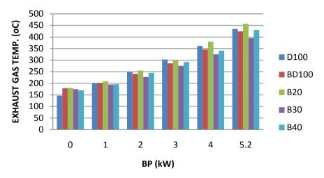
Figure 5. Exhaust gas temperature with BP.
