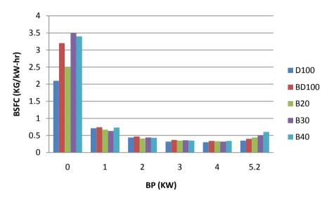
Figure 3. Brake specific fuel consumption with BP.
