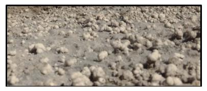
Figure 6. Salt deposition by evaporation of brine.
