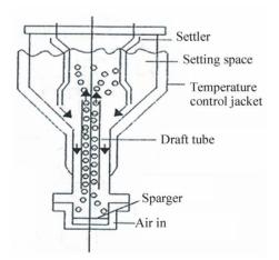
Figure 9. Airlift loop reactor with draft tube as riser.
