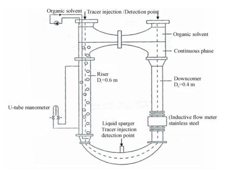
Figure 7. Liquid impelled loop reactor (LILR).
