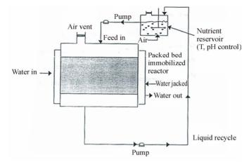
Figure 12. Packed bed reactor.
