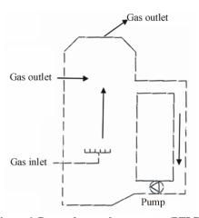
Figure 6. Pumped tower loop reactor (PTLR).
