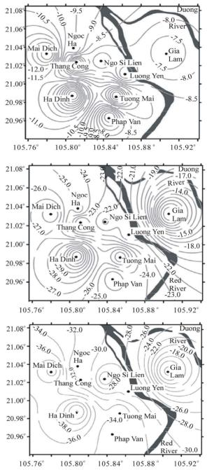
Figure 2. Groundwater levels in some districts of Hanoi in 1993 (top), 2005 (middle), and 2020 (bottom) (prognosis based on data from 1993 and 2005).
