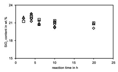
**Figure 5.** Silica content of liquid phases prepared from batch A as a function of dissolution time; dissolution temperatures:  $\Box$ : 160°C,  $\diamond$ : 200°C,  $\Delta$ : 220°C.
