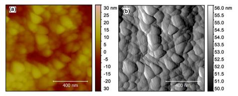
**Figure 4.** Atomic force microscope image of opal fracture surface; (a) height image, (b) tapping amplitude image measured for structure analyzation; lateral scale bar in the picture, height or deflection scale on right side.
