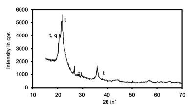
**Figure 2.** X-ray diffraction pattern of opal; CuK*a* radiation; t: tridymite (JCPDS 18-1170), q: low-quartz (JCPDS 2-458).
