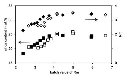
**Figure 8.** Silica content ( $\blacksquare$ : batch D,  $\square$ : batch E) and measured values of  $R_m$  ( $\blacklozenge$ : batch D,  $\diamondsuit$ : batch E) of liquid phases as a function of the initial  $R_m$  value; dissolution time 6 h; dissolution temperature 160°C.
