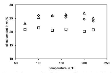
**Figure 7.** Maxima of silica contents of liquid phases prepared from batches B ( $\diamond$ ) and C ( $\Delta$ ) as a function of dissolution temperature; dissolution times 4 h or 6 h; final value of silica content of liquid phase prepared from batch A ( $\Box$ ) at that these temperatures included for comparison.
