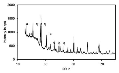
**Figure 9.** X-ray diffraction pattern of solid residue after hydrothermal treatment of opal in NaOH lye; batch B, dissolution temperature: 220°C; dissolution time: 20 h; nonalkaline oxide content: 18.5 wt.%, Na<sub>2</sub>O: 7.8 wt.%,  $R_m = 2.44$ ; CuK*a* radiation; a: analcime (Na[AlSi<sub>2</sub>O<sub>6</sub>]·H<sub>2</sub>O; JCPDS 2-340), q: low-quartz (JCPDS 2-458).
