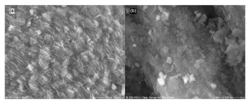
**Figure 3.** Electron micrographs of common opal; scale bar in the lower right corner; (a) surface inside larger pore, (b) fracture surface.
