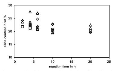
**Figure 6.** Silica content of liquid phases prepared from batches A ( $\Box$ ), B ( $\diamondsuit$ ), and C ( $\Delta$ ) as a function of dissolution time; dissolution temperature 200°C.
