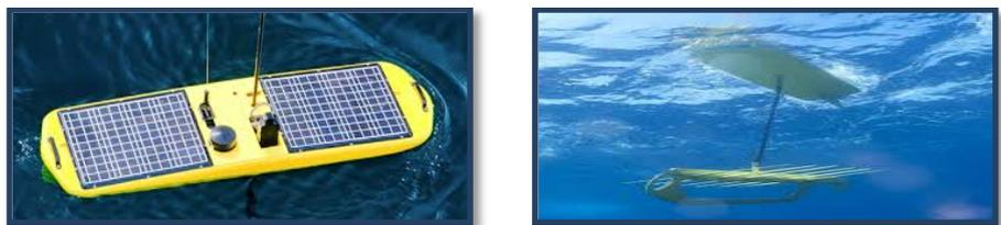
**Figure 1.** wave glider showing the surface vehicle and submerged glider ([www.bing.com/images/waveglider](http://www.bing.com/images/waveglider)).
