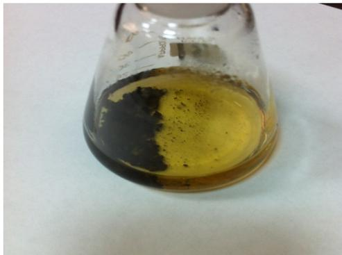
**Figure 1.** Purification process of synthesized MWCNTs in the xylene.
