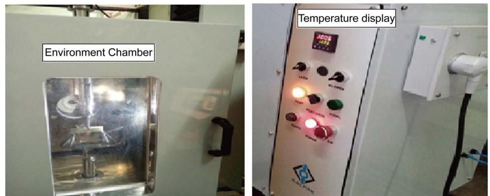
**Figure 2.** Universal testing machine showing the sample position at elevated temperature.
