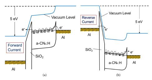
**Figure 22.** Energy band diagrams in (a) forward (left), and (b) reverse (right) current statuses of the I-V curves (Al/SiO<sub>2</sub>/a-CN<sub>x</sub>:H/Al).
