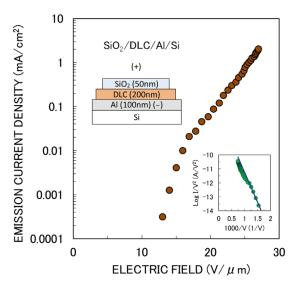
**Figure 8.** Emission current-voltage characteristics of SiO<sub>2</sub>/a-CN<sub>x</sub>:H/Al/Si structure. a-CN<sub>x</sub>:H film was deposited at 100/800W. Insets show layer structure and FN plot.
