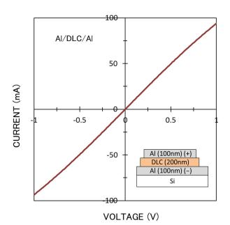
Figure 9. I-V characteristic of Al/a-CN<sub>x</sub>:H/Al structure. Inset shows the layer structure.
