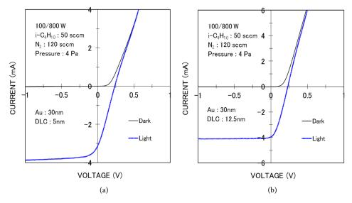
**Figure 17.** I-V characteristics of a-CN<sub>x</sub>:H/p-Si PVCs measured in dark and light. a-CN<sub>x</sub>:H thicknesses of (a) 5 (left), and (b) 12.5 (right) nm.
