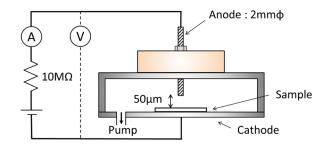
Figure 6. Schematic of field emission measurement apparatus with 50-µm space between anode and sample.
