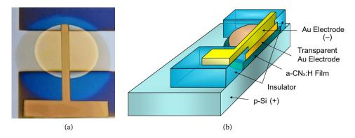
Figure 15. (a) Photograph (left), and (b) structure (right) of fabricated Au/a-CN<sub>x</sub>:H/p-Si PVC.
