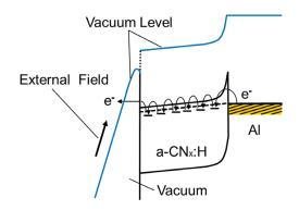
Figure 24. Energy band diagram in electron field emission situation of the a-CN<sub>x</sub>:H/Al device.
