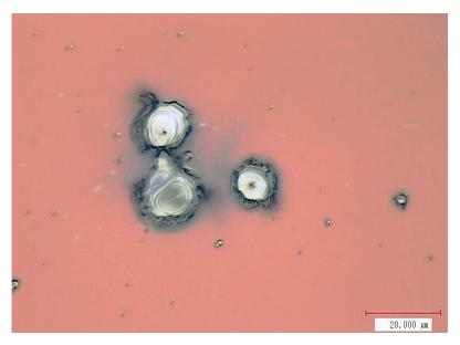
Figure 13. Photograph of craters formed by the vacuum arc discharge at emission sites.
