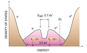
Figure 20. Schematic representation of density of states (DOS) in 100/800W a-CN<sub>x</sub>:H film.
