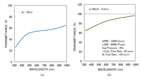
Figure 16. Transmittances of (a) 30-nm thick Au electrode (left); (b) 12.5-nm thick a-CN<sub>x</sub>:H (right).
