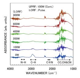
**Figure 5.** FTIR absorption spectra of a-CN<sub>x</sub>:H films as a function of LORF (0 - 800 W). UPRF was 100 W. Used gases were i-C<sub>4</sub>H<sub>10</sub> (50 sccm) and N<sub>2</sub> (120 sccm).
