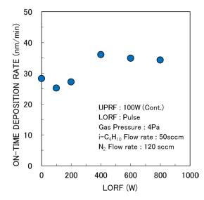
Figure 2. LORF (0 - 800 W) dependence of the on-time deposition rate measured at UPRF of 100 W.
