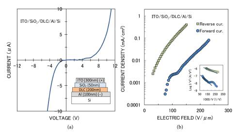
**Figure 12.** (a) I-V characteristic (left); (b) semi-log plot of I-V curve (right) of ITO/SiO<sub>2</sub>/a-CN<sub>x</sub>:H/Al structure. Inset shows (a) layer structure, and (b) FN plot.
