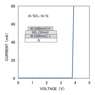
Figure 10. I-V characteristic of Al/SiO<sub>2</sub>/Al structure. Inset shows the layer structure.
