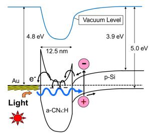
Figure 25. Energy band diagram in photovoltaic situation of a-CN<sub>x</sub>:H/p-Si PVC.
