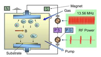
We used a PRF SMP CVD apparatus under RF power modulated by a 2.5-kHz pulse
