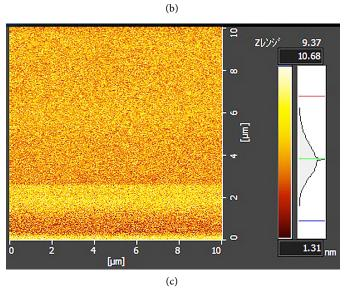
**Figure 14.** Surface morphology of (a) a-CN<sub>x</sub>:H/Al/Si (upper); (b) a-CN<sub>x</sub>:H/Al/glass (middle); (c) Al/SiO<sub>2</sub>/a-CN<sub>x</sub>:H/Al/Si (lower) measured using AFM. Observation area was  $5 \times 5$  or  $10 \times 10 \ \mu m^2$ .
