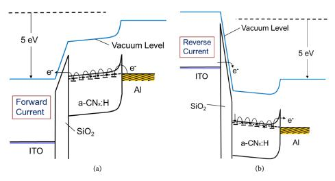
**Figure 23.** Energy band diagrams in (a) forward (left), and (b) reverse (right) current statuses of the I-V curves (ITO/SiO<sub>2</sub>/a-CN<sub>x</sub>:H/Al).
