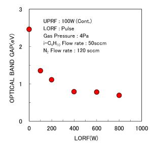
Figure 3. Optical band gap of a-CN<sub>x</sub>:H films as a function of LORF (0 - 800 W). UPRF was 100 W.
