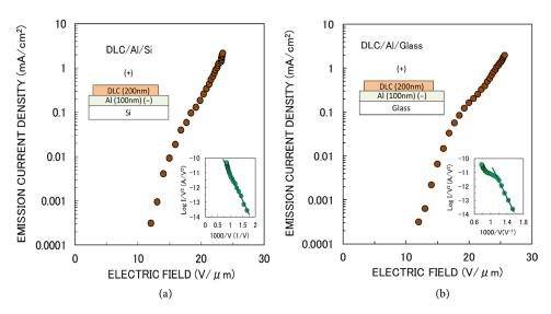
**Figure 7.** (a) Emission current-voltage characteristics of a-CN<sub>x</sub>:H film deposited at 100/800 W on (a) Al/Si (left), and (b) Al/glass (right) substrates. Insets show layer structures and FN plots.
