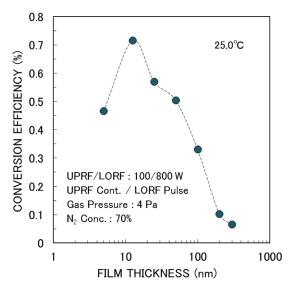
**Figure 18.** Conversion efficiency of a-CN<sub>x</sub>:H/p-Si PVCs with a-CN<sub>x</sub>:H films about 5 - 300 nm-thick.
