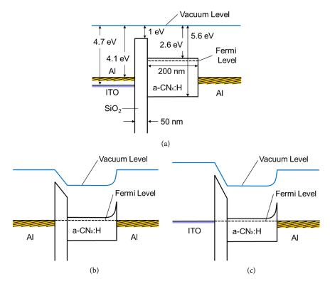
**Figure 21.** Proposed energy band diagrams of Al/SiO<sub>2</sub>/a-CN<sub>x</sub>:H/Al and ITO/SiO<sub>2</sub>/a-CN<sub>x</sub>:H/Al structures. (a) flat-band (upper), thermal equilibrium band diagram of (b) Al/SiO<sub>2</sub>/a-CN<sub>x</sub>:H/Al (lower left); (c) ITO/SiO<sub>2</sub>/a-CN<sub>x</sub>:H/Al (lower right).
