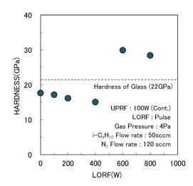
Figure 4. Hardness of a-CN<sub>x</sub>:H films as a function of LORF (0 - 800 W). UPRF was 100 W.
