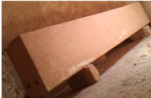
**Figure 2.** A view of a baked clay beam after firing in Potter's type kiln.
