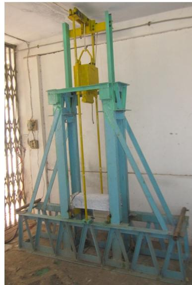
**Figure 4.** A reinforced baked clay beam of dimensions 150 mm × 150 mm × 500 mm is being tested for drop weight impact loading.
