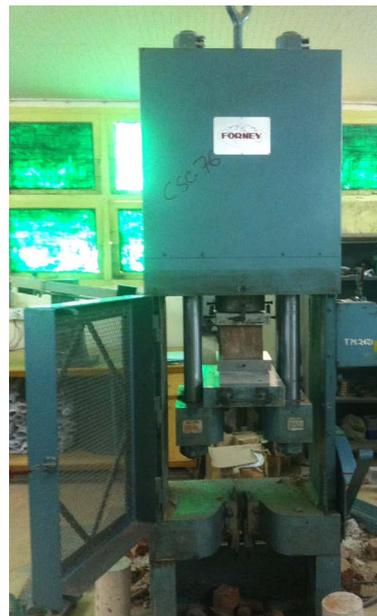
**Figure 3.** Determination of compressive strength of a baked clay cube in Universal Testing Machine.
