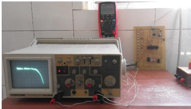
**Figure 14.** Curves I-V characteristic in the static mode under illumination polychromatic at 39°C under an ambient temperature of 33.5°C.
