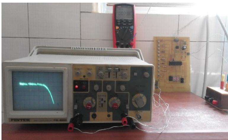
**Figure 17.** Curves I-V characteristic in the static mode under illumination polychromatic at 45°C under an ambient temperature of 33.8°C.
