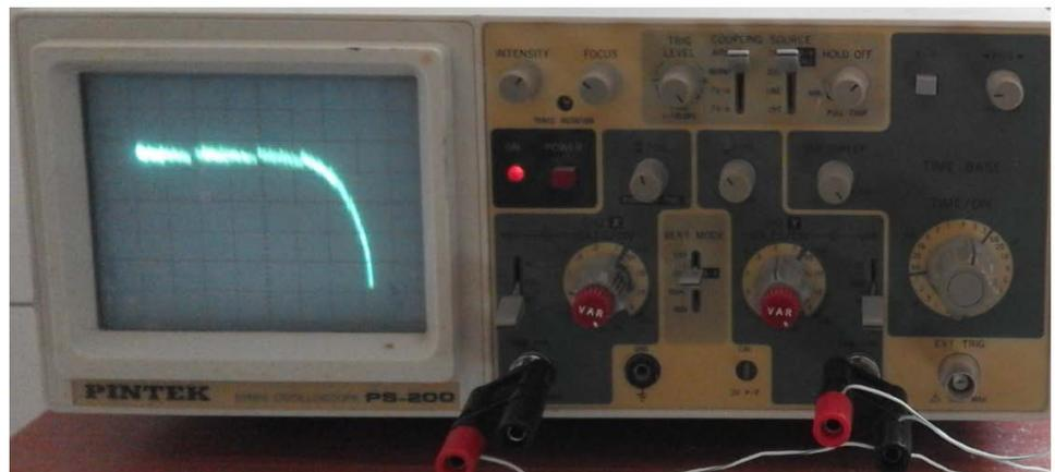
**Figure 18.** Curves I-V of the solar panel for polychromatic illumination.
