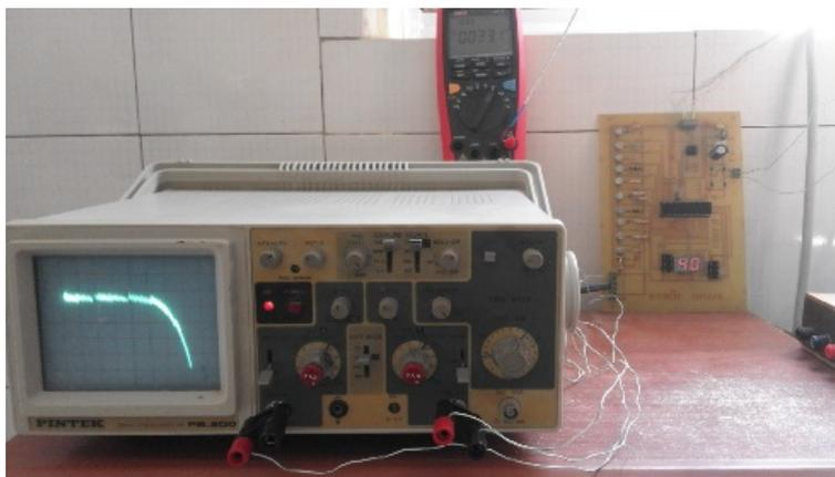
**Figure 15.** Curves I-V characteristic in the static mode under illumination polychromatic at 40°C under an ambient temperature of 33.1°C.
