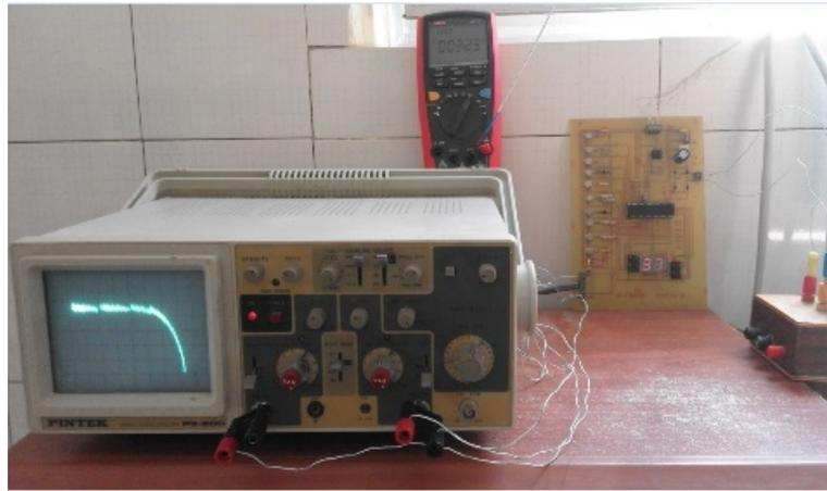
**Figure 12.** Curves I-V characteristic in the static mode under illumination polychromatic at 37°C under an ambient temperature of 32.3°C.
