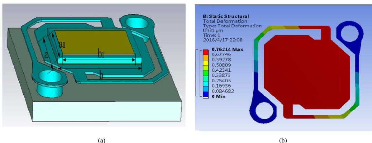
**Figure 2.** (a) The model of microbolometers in simulation; (b) simulated deformation of the microbridge.
