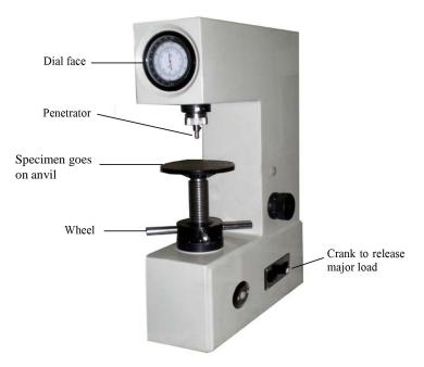
Figure 3. Major components of a Rockwell hardness tester [4].
