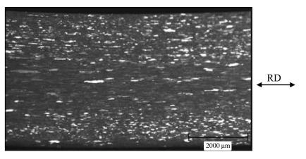
**Figure 6.** Macrograph of sample taken from coupon 3, partially annealed rolled (AA6061 H13). As etched with Poulton's reagent.
