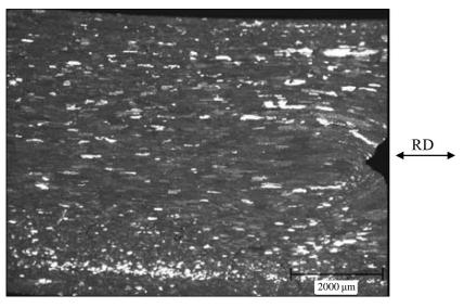
**Figure 4.** Macrograph of sample taken from coupon 1, "fully" rolled (AA6061 H16). As etched with Poulton's reagent.
