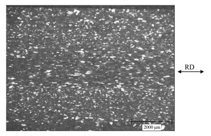
**Figure 5.** Macrograph of sample taken from coupon 2, fully annealed (AA606-O). As etched with Poulton's reagent.
