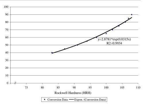
**Figure 7.** Hardness conversion from Rockwell H Scale to Standard Brinell Hardness. The graph was constructed based on numbers from literature.
