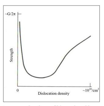
Figure 1. Strength as a function of dislocation density [5].
