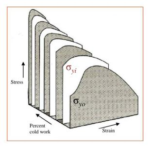
**Figure 2.** Increasing %CW increases stress ( $\sigma$  represents the strain) [8].
