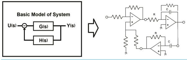
Figure 5. Basic feedback system and the equivalent electronic circuit [3].
