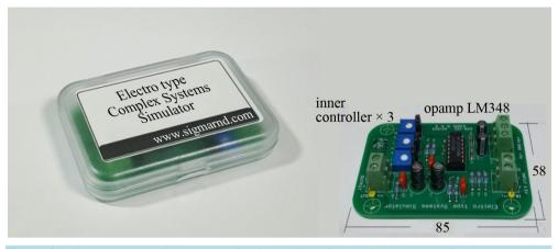
Figure 2. Electrotype complex systems simulator (50% size) and the system simulator prototype (available eBay).
