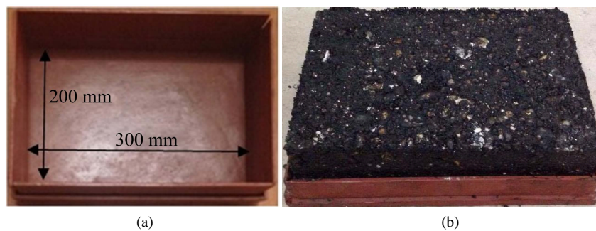
Figure 5. The parts of the used mould of specimen. (a) Complete mould; (b) Mould with specimen after removing upper part.
