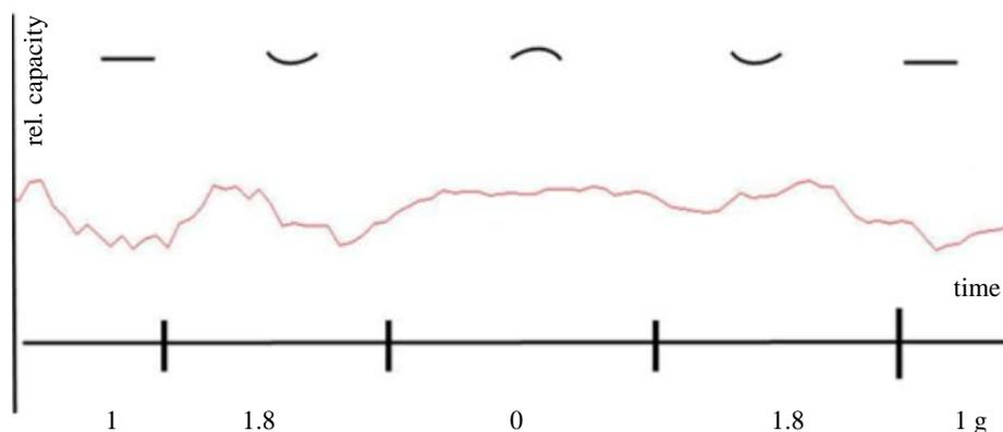
**Figure 3.** Capacity changes of a bilayer depending on gravity in a parabolic flight. Changes are not significant. Possibly there is a small effect of gravity on bilayer curvature as sketched above the trace.
