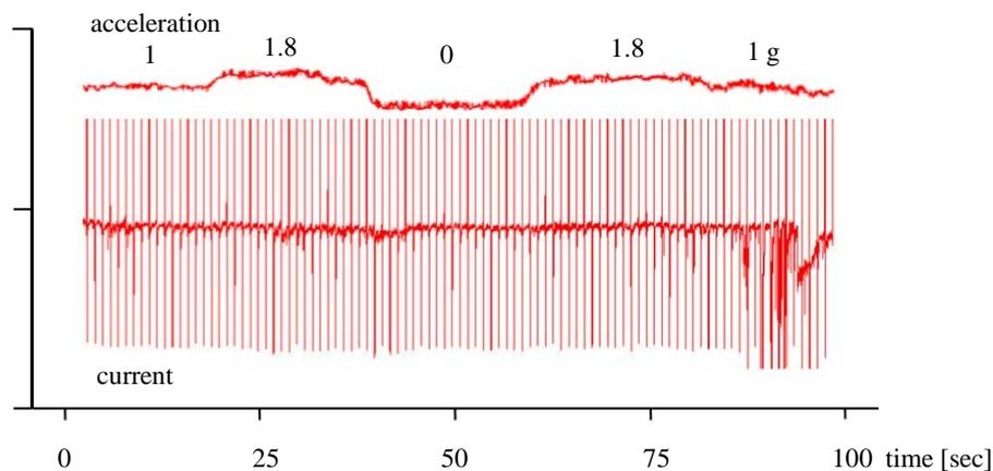
**Figure 2.** Current recording from an asolectin bilayer at 120 mV with superimposed pulse-protocol for capacity recording. To give a better assignment to the gravity level, a smoothed recording of the actual gravity level of the used parabola is given above the current recording.
