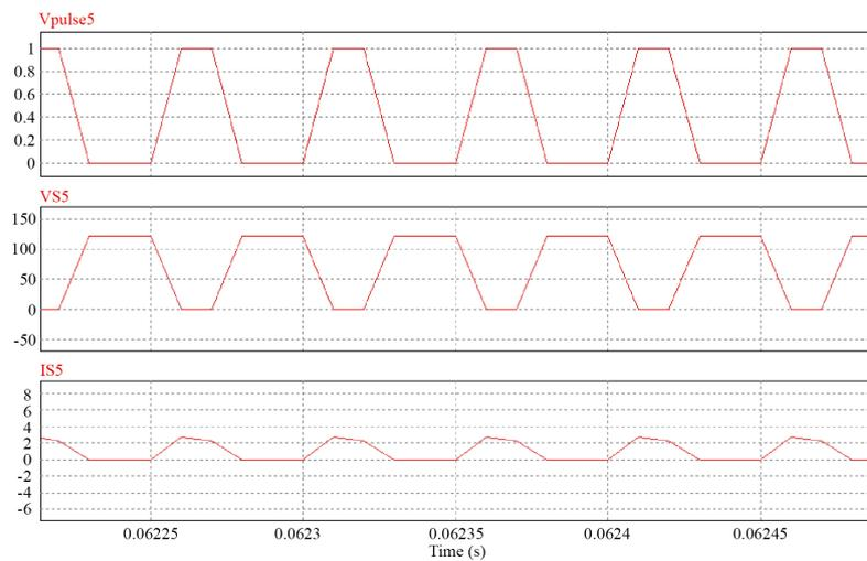
Figure 5. The switching pulses, voltage across the switch and switch currents for S5 & S6.
