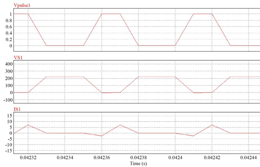
Figure 6. The switching pulses, voltage across the switch and switch currents for S7 & S8.
