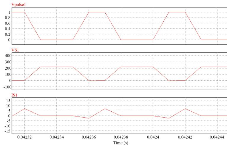
Figure 3. The switching pulses, voltage across the switch and switch currents for S1 & S2.
