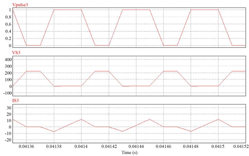
Figure 4. The switching pulses, voltage across the switch and switch currents for S3 & S4.
