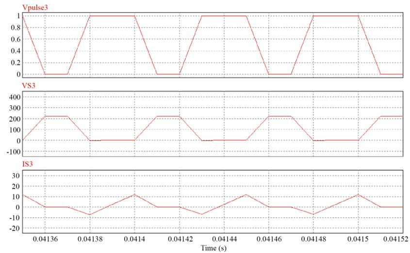
Figure 7. Zero Current Zero Voltage Switching of switches.
