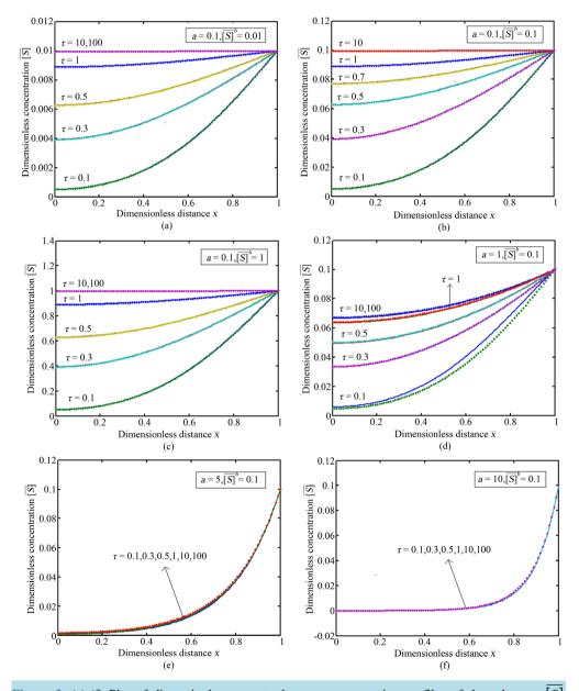
Figure 3. (a)-(f) Plot of dimensionless non-steady state concentration profiles of the substrate [S] versus dimensionless distance  $\overline{x}$  for fixed values of *a* and  $\overline{[S]}^{b}$  and various values of time  $\tau$ . Solid lines represent the Equation (15) and the dotted lines represent the numerical simulation.
