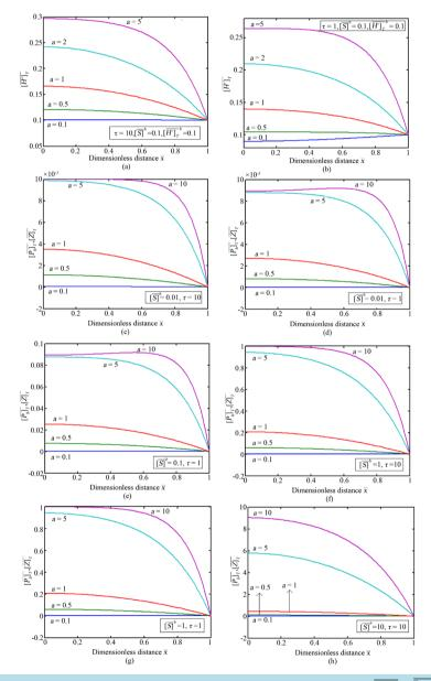
Figure 6. (a)-(h) Plot of dimensionless non-steady state concentration profiles of products  $\overline{[Z]}_{T}$ ,  $\overline{[H^+]}_{T}$  and  $\overline{[P_h]}_{T}$  versus dimensionless distance  $\overline{x}$  for fixed values of  $\overline{[S]}^{b}$  and  $\tau$  and various values of the parameter *a* using Equations (16), (17) and (18).
