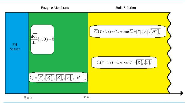
Figure 2. Boundary conditions employed in the pH-based potentiometric biosensor for the substrate [S], products  $[P_h]_T, [\overline{Z}]_T, [\overline{H^+}]_T$  and added external buffer concentration of species (AH)  $[\overline{A}]_T$ .
