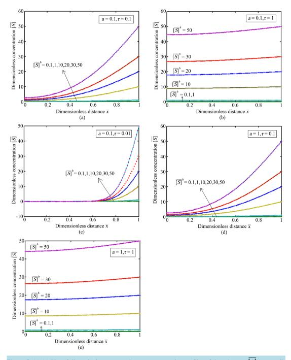
Figure 5. (a)-(e) Plot of dimensionless non-steady state concentration profiles of the substrate [S] versus dimensionless distance  $\overline{x}$  for fixed values of *a* and time  $\tau$  and various values of the parameters  $\overline{[S]}^{b}$ . Solid lines represent the Equation (15) and the dotted lines represent the numerical simulation.
