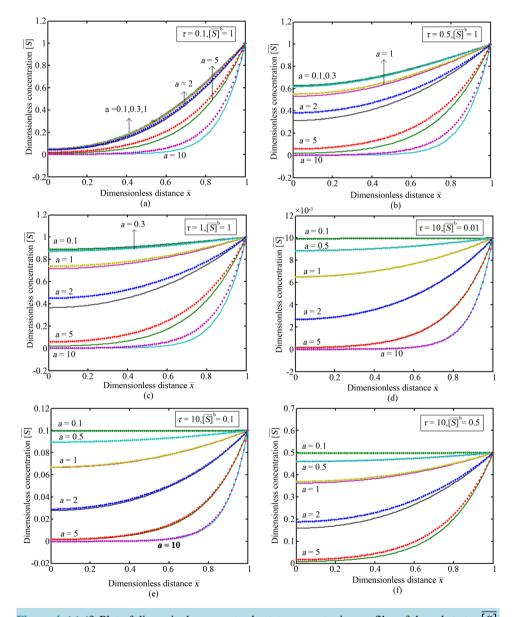
Figure 4. (a)-(f) Plot of dimensionless non-steady state concentration profiles of the substrate [S] versus dimensionless distance  $\overline{x}$  for fixed values of time  $\tau$  and  $\overline{[S]}^{b}$  and various values of the parameters *a*. Solid lines represent the Equation (15) and the dotted lines represent the numerical simulation.
