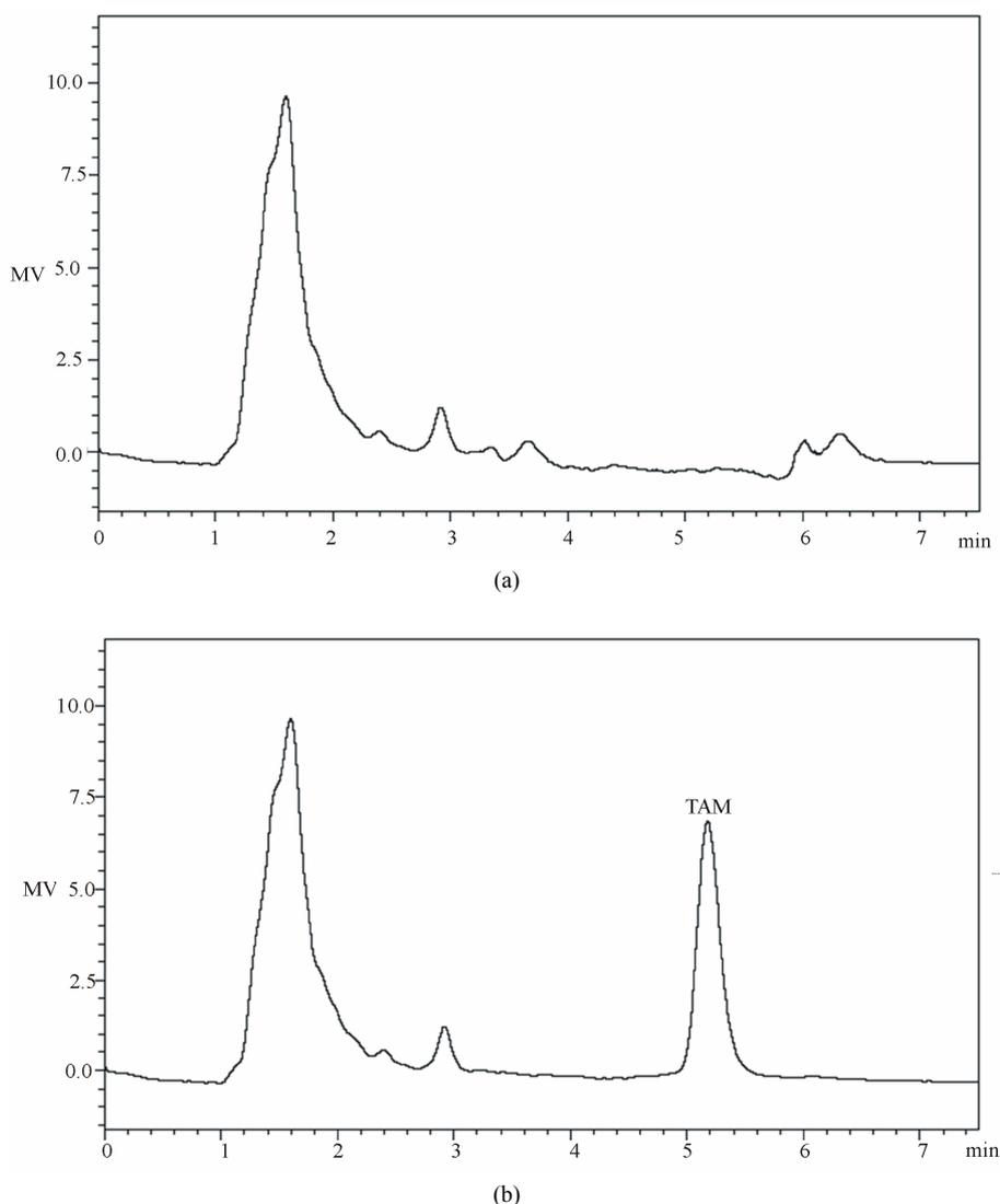
**Figure 4.** The chromatograms of (a) non-spiked plasma samples with TAM under the optimum conditions, and (b) the spiked (at the concentration level of  $25.0 \text{ ng}\cdot\text{mL}^{-1}$ ).
